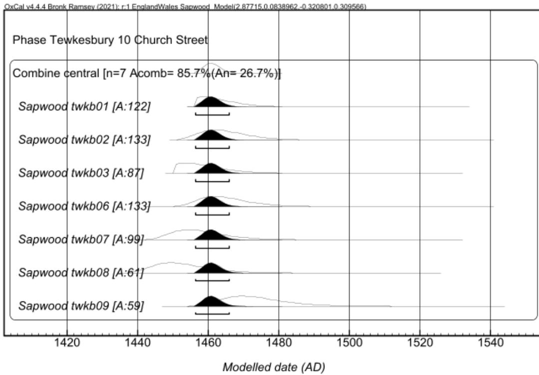
Figure 6: Probability distributions for the date of the felling of timbers from the central bay. Individual felling date distributions are shown in outline and the combined felling date distribution is shown in black with the 95.4% probability range bar below.
