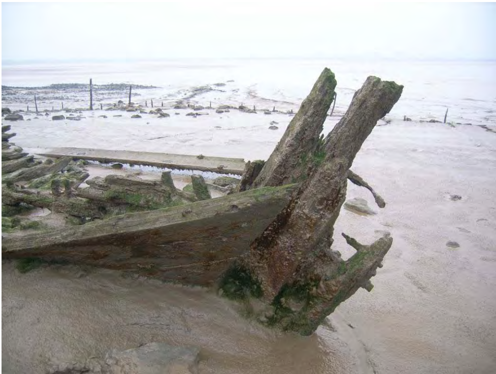
Plate 230: The sternpost, lower hull and part of the rudder of another hulked vessel at Lydney, Glos. ( Line No. 40006 ).
