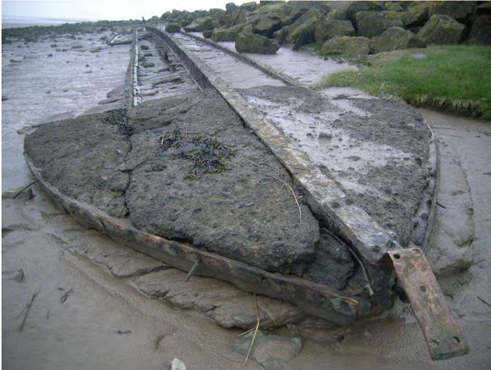
Plate 229: The hulk of a wooden and iron vessel south-west of Lydney harbour, Glos. ( Line No. 40053 ). Note the concrete infill of the lower hull.
