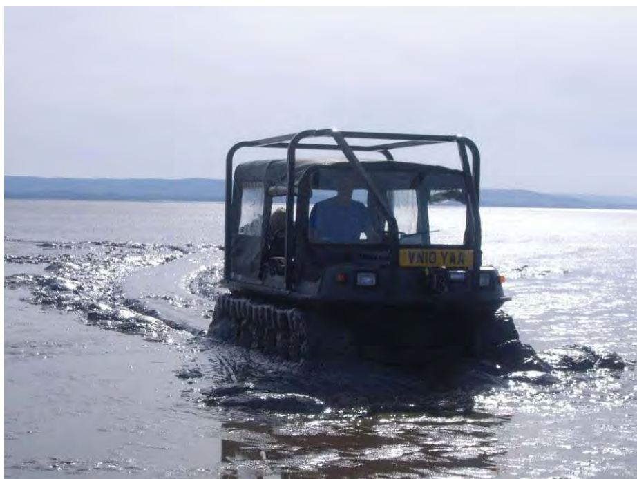
Plate 4: The first deployment of the Argocat off Brean/Berrow Beach, Somerset, where the vehicle became bogged down only c. 20m from the edge of firmer sand. Nick Witchell was fortunately able to extricate it from the deep, liquid sucking mud.
