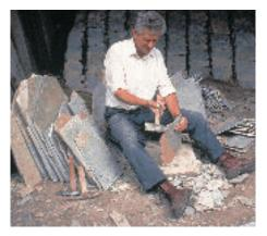
**Figure 5** Once split to a suitable thickness, the stone is dressed roughly square and a fixing hole made.
