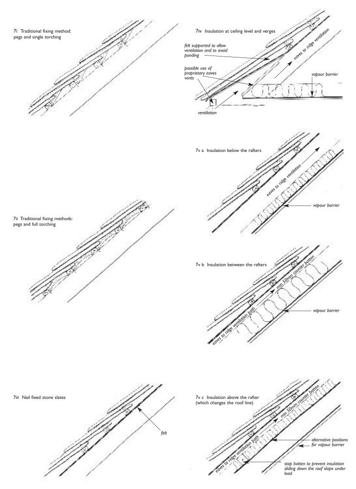
Figure 7 Fixing methods and the use of different types of torching and roofing felts for stone slating
