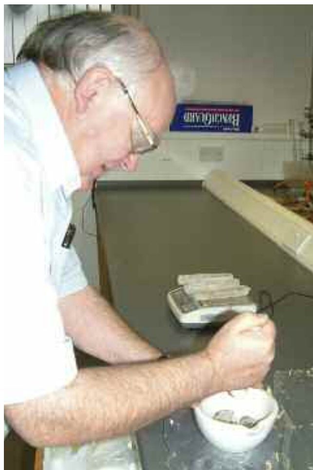
Fig 14. Robert Anderson homogenising a bulk sample of peat at the Scottish Universities Research and Reactor Centre. (© Historic England, photography by Amanda Grieve)
