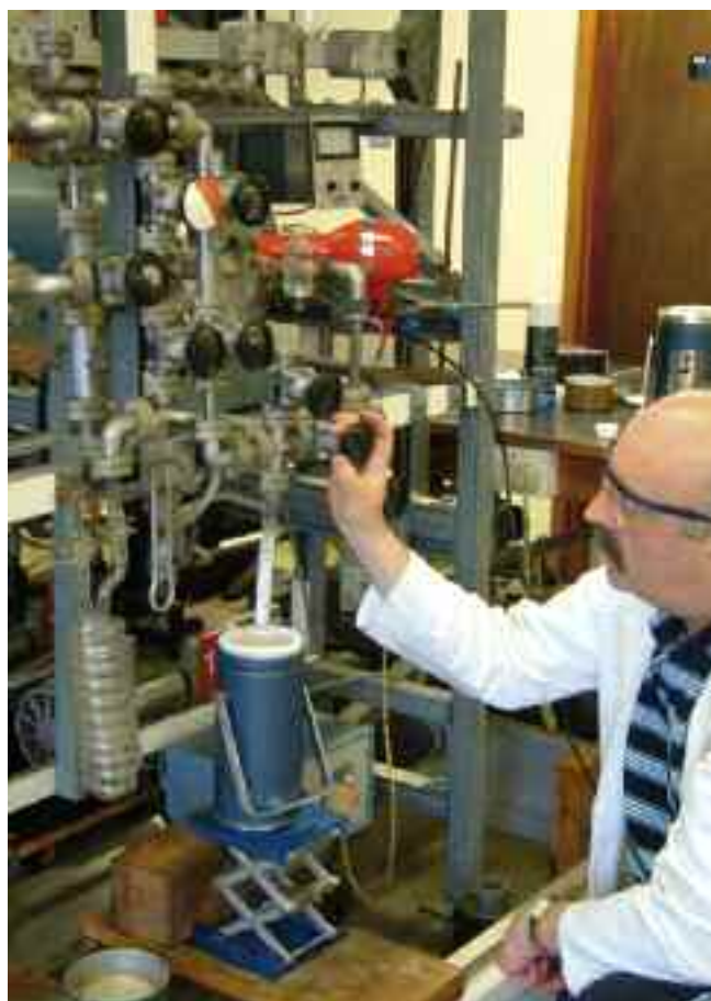
Figure 15. James MacDonald preparing benzene at the Queen's University, Belfast radiocarbon laboratory (© Historic England, photography by Amanda Grieve)
