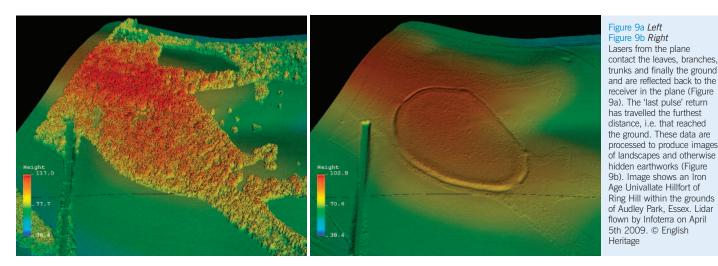
Airborne remote sensing - lidar
