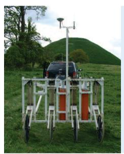
Figure 8 Towed magnetometer array consisting of two SQUID gradiometers with integral GPS system. Photo courtesy of Neil Linford. © English Heritage.
