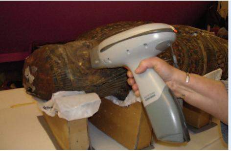
Figure 19 Portable XRF analysis of an Egyptian cartonnage for display at Brighton Museum. Image courtesy of Dana Goodburn-Brown.
