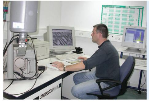
SEM examination and EDS analysis of copper alloy slag from a 17th-century context in Colchester. The analysis showed that the alloy used was of the sort used in the manufacture of cauldrons (not bells). © English Heritage.
