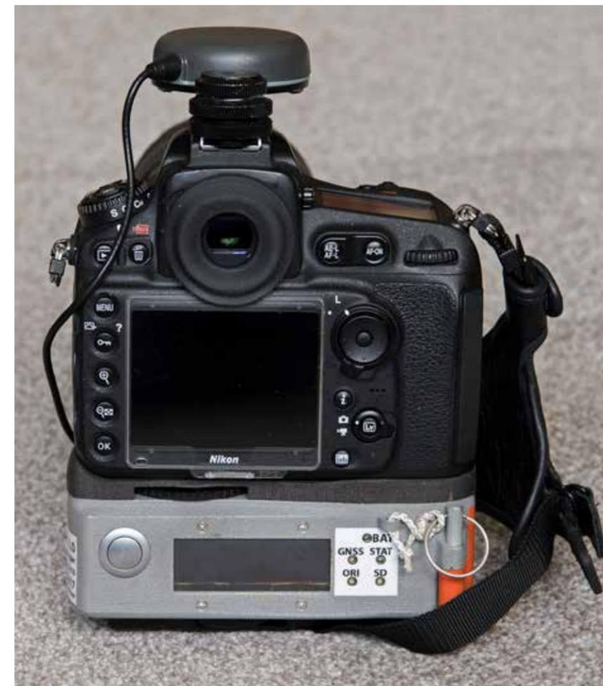
**Left:** The Inertial Navigation System, developed by Martin Weiser at the University of Vienna, attached to our Nikon camera. This allows us to import the footprint of each photograph into our geographical information systems (GIS).
