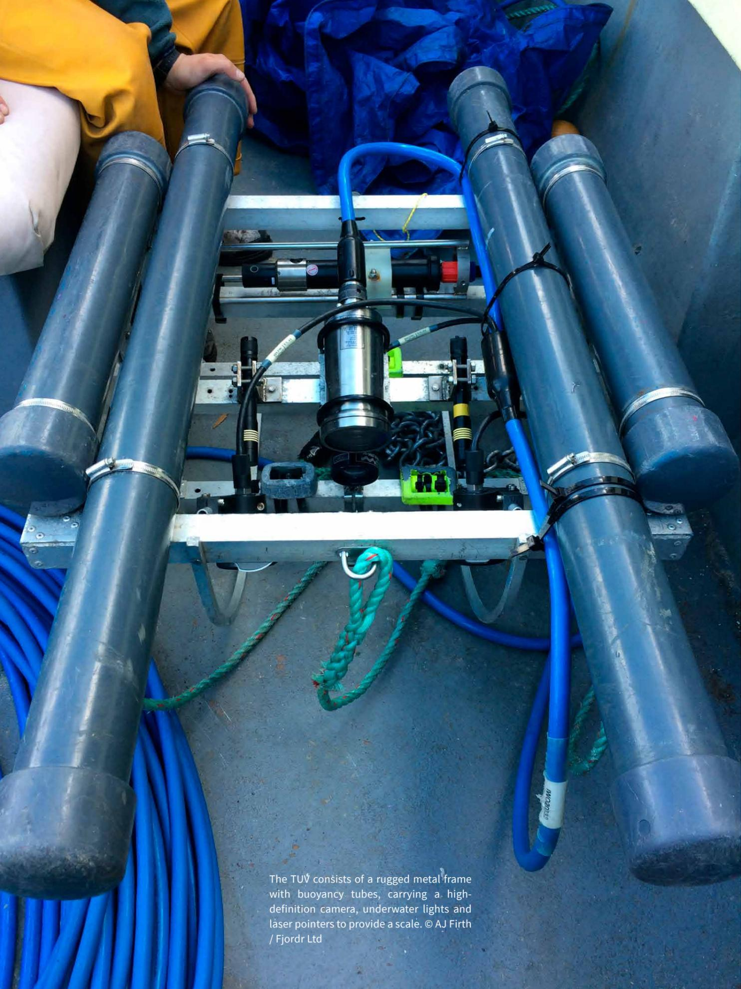
The TUV consists of a rugged metal frame with buoyancy tubes, carrying a high-definition camera, underwater lights and laser pointers to provide a scale. © AJ Firth / Fjordr Ltd
