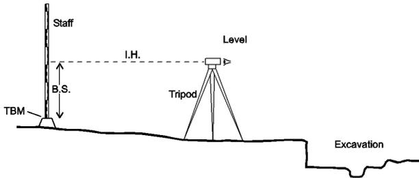
Then take a Foresight (FS) reading with the staff on the points you want to level (but never directly on a find!). The height OD of the target point (its Reduced Level or RL) is the Instrument Height minus the Foresight.
