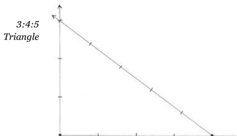
Set up a suitable baseline, and then use 30m tapes to set out a right angle using the 3:4:5 triangle method. Make the triangle as large as possible (e.g. 15:20:25 metres rather than 3:4:5 metres) as extending lines out from a small triangle is likely to be inaccurate.
