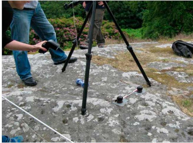
**Tip:** Tripod legs sometimes create unwanted shadow during a capture sequence. If available, a copy stand can be used to stabilise the camera and eliminate additional sources of shadow.
