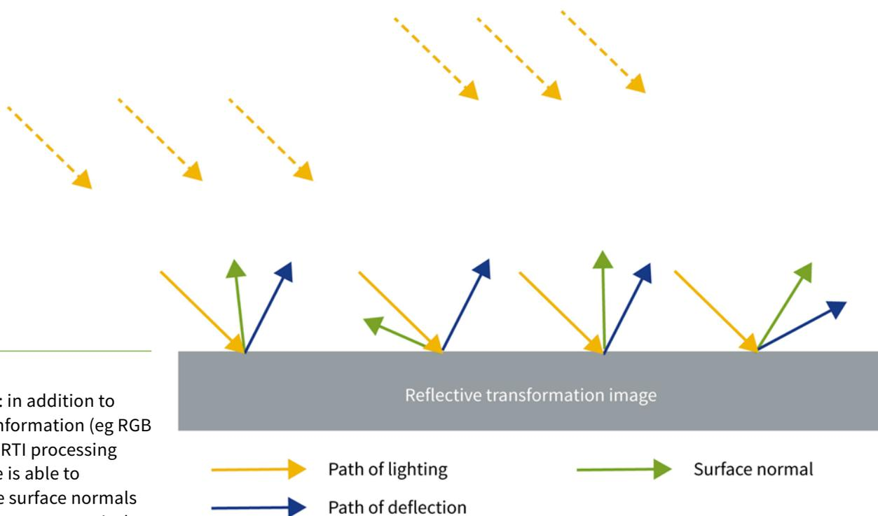
Figure 3: in addition to colour information (eg RGB values), RTI processing software is able to estimate surface normals of an image set per pixel. The surface normal data provide information about the 3D shape of the surface. © Sarah M Duffy
