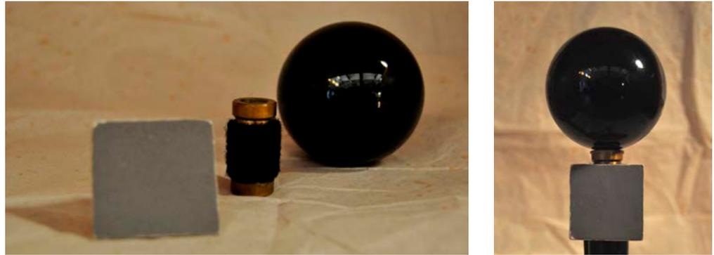
a tripod might not be necessary for placing the target(s). In such instances, the target can be mounted on a stable item, such as the bottom of a flat, rubber end-cap and placed next to the subject (as in Fig 8).
