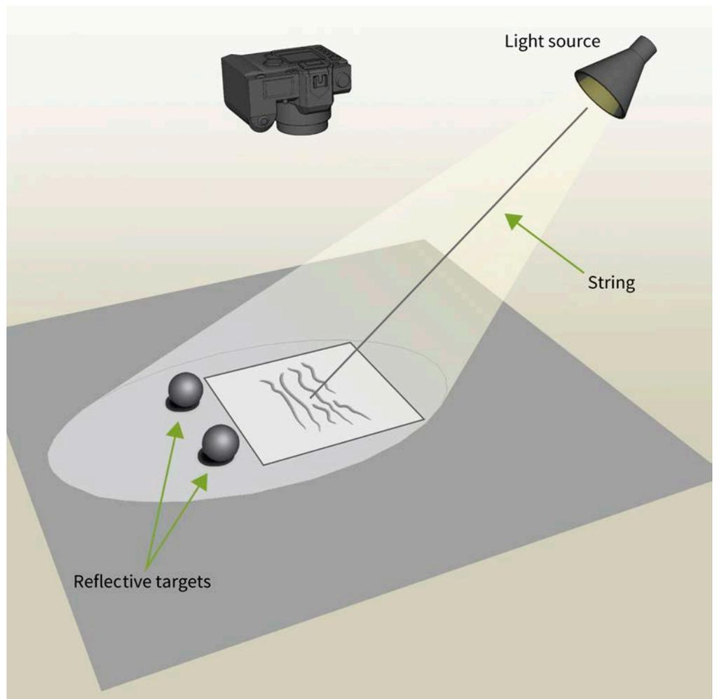
In order to optimise the reflectance information, additional ambient lighting – such as overhead lights or sunlight – should be controlled. This can be achieved by recording in a dark room or use specialised filters. In the post-processing phase, a certain degree of adjustment can be made to the image set before they are fed through the specialised software that produces an interactive RTI file.
