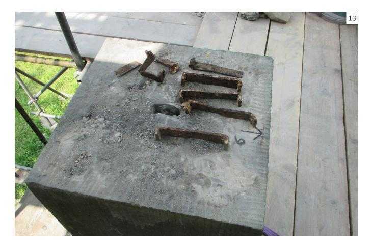
**Figure 13**Corroded cramps at Waterloo Memorial, Billinge, Merseyside.
