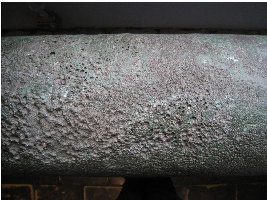
Plate 3: minor patches of active corrosion (pale areas) on Gun 1
