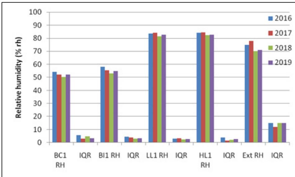
Fig 64: January/February median humidity (%) and interquartile ranges (IQR) in the room (BC), below insulation (BI), Roof 1 (HL and LL) and the exterior (Ext) for 2016 to 2019
