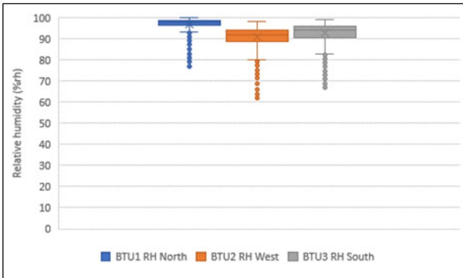
Fig 5: Relative humidity (%) under the tiles for different roof slope orientations. The humidity under the north slope is the highest and least variable
