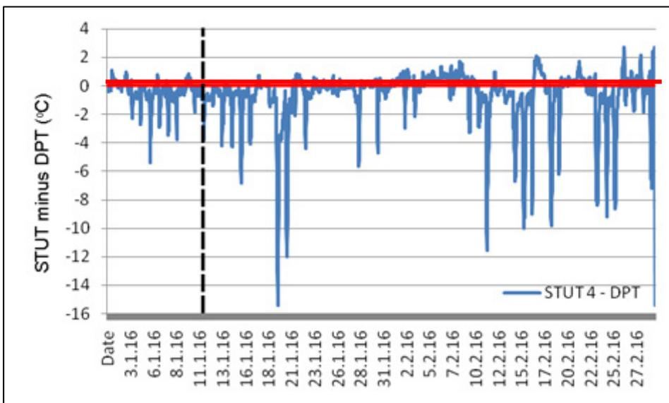
Fig 10: Condensation risk (under red line) in west corner of roof January/February 2016 obtained by subtracting dew point temperature (DPT) from surface temperatures under tiles (STUT). The dotted line is the date occupancy commenced
