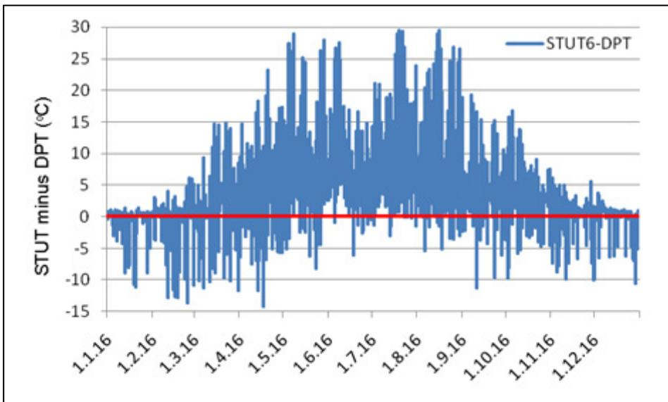
*Fig 45: The condensation risk (below red line) shows seasonal trends during 2016 obtained by subtracting the dew point temperature (DPT) beneath the tiles and underlay from the surface temperature of the underside of the tiles (STUT)*
