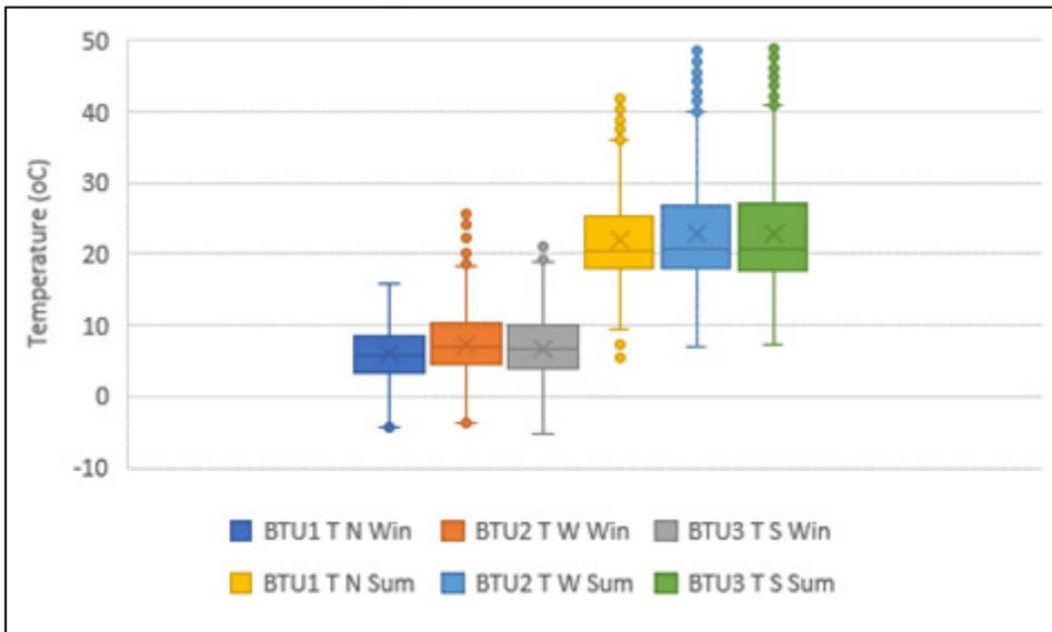
Fig 36: A comparison of winter (Win) and summer (Sum) air temperatures (°C) for the space between the tiles and the underlay (BTU) during 2016
