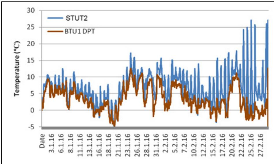
Fig 60: Surface temperature (STUT2) compared with dew point temperature (DPT) for January/February 2016
