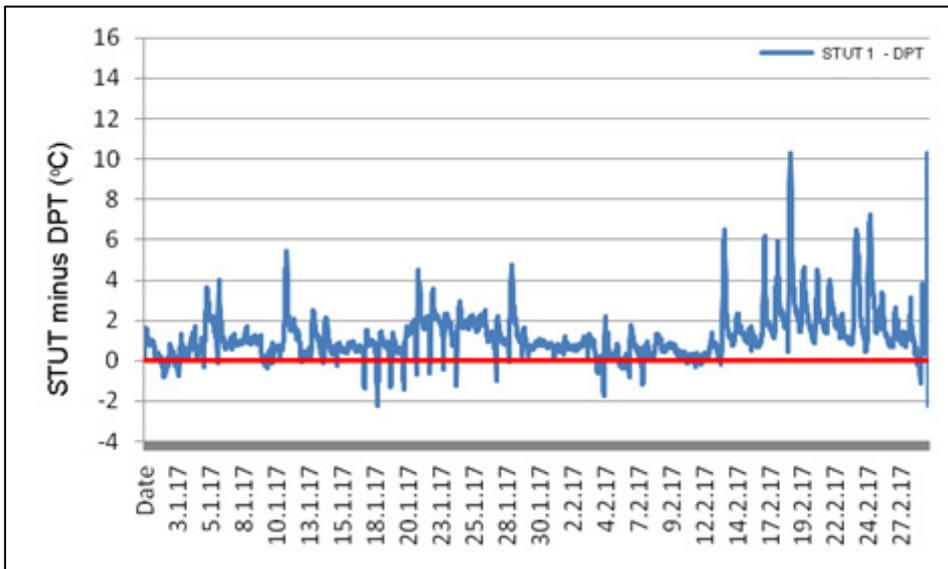
Fig 86: Condensation risk (below red line) on the north slope for January/February 2017 obtained by subtracting dew point (DPT) from surface temperature under tiles (STUT). The thickness of insulation was 300mm
