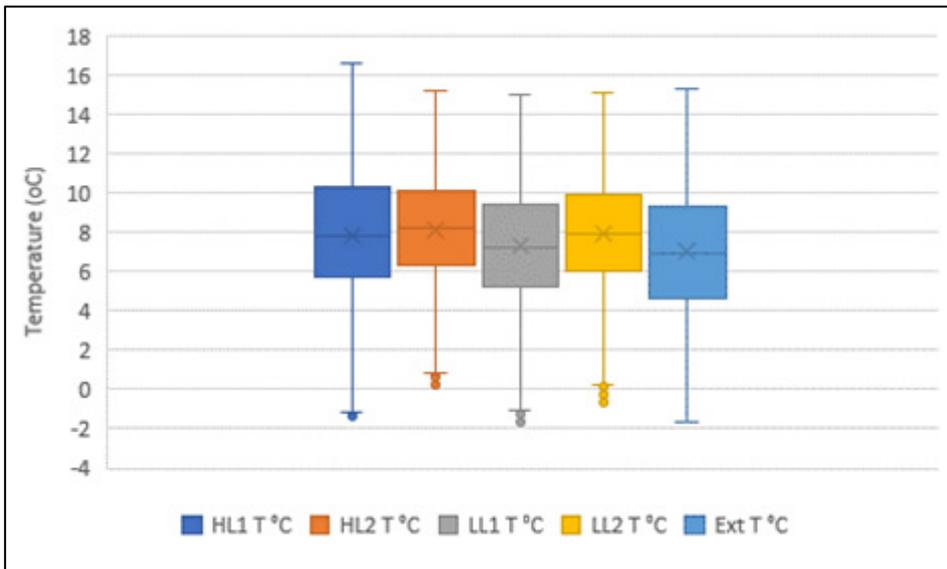
Fig 53: January/February median temperatures (°C) at high (HL) and low (LL) levels, with their interquartile ranges compared with exterior (Ext) for 2016
