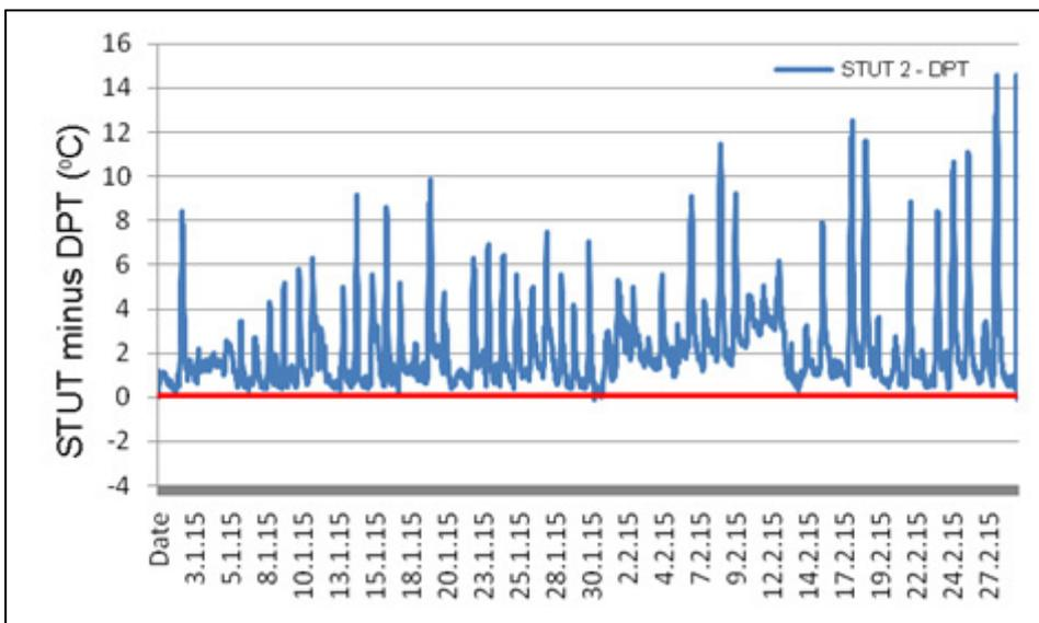
Fig 83: Condensation risk (below red line) on the south slope for January/February 2015 obtained by subtracting dew point (DPT) from surface temperature under tiles (STUT). There was 100mm of insulation between the joists
