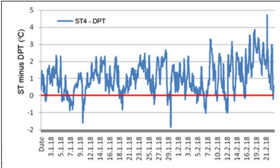
Fig 121: January/February 2018 condensation events (below red line) for the north slope of the roof
