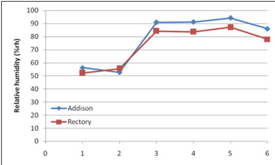
Fig 143: The average relative humidity gradients across the roof from the room (1) to the exterior (6) during the first week of January 2017
