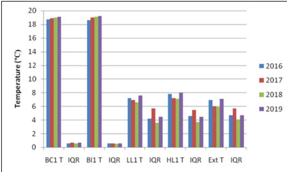
Fig 62: January/February average temperatures (°C) and interquartile ranges (IQR) in the room (BC), below insulation (BI), Roof 1 (HL and LL) and the exterior (Ext) for 2016 to 2019
