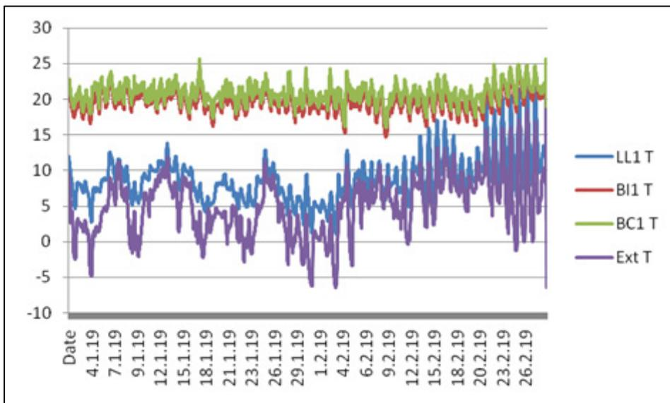
*Fig 132: The room (BC) and below insulation (BI) environments remain much warmer than the roof above the insulation (LL) and the exterior (Ext). There is no indication that occupancy during January and February warms the roof space*
