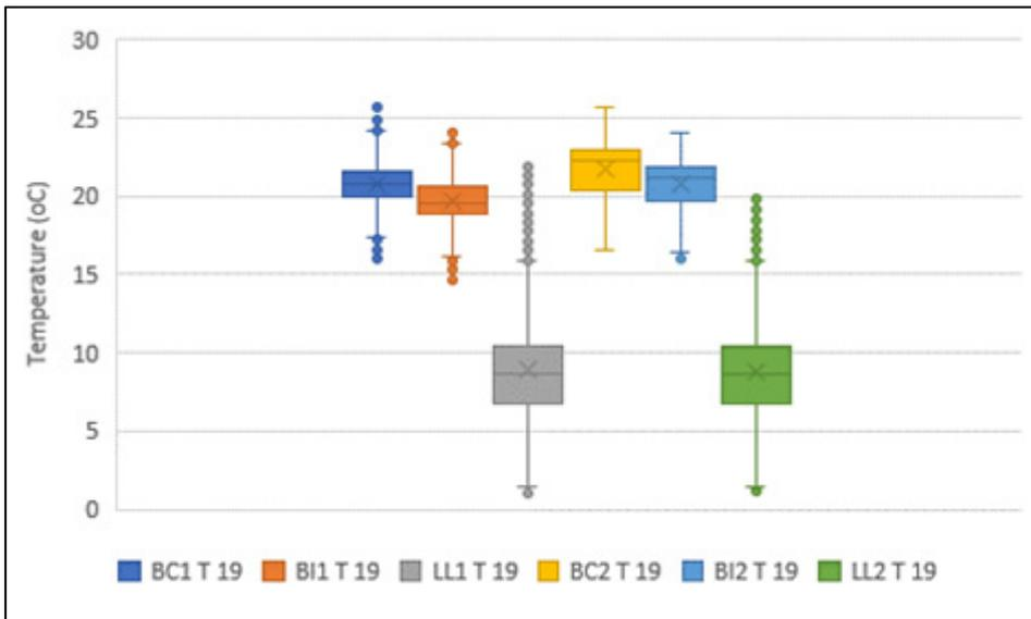
Fig 128: Temperature gradients (°C) from below ceiling (BC) to low level (LL) in the roof for January/February 2019. BC1 is in a spare unused bedroom; BC2 is in the bathroom
