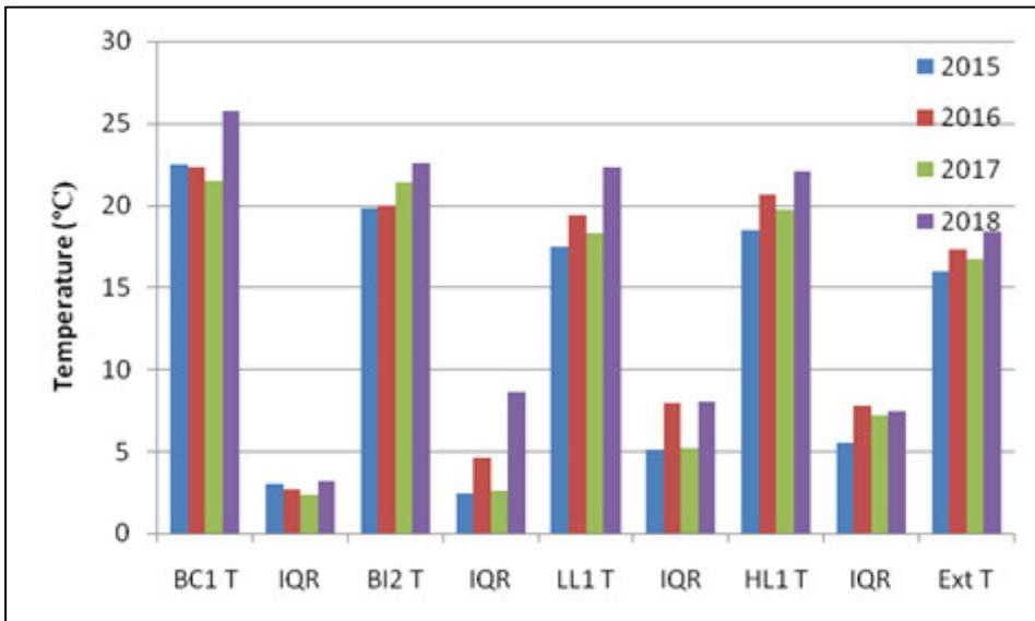
Fig 104: July/August average temperatures (°C) in the room (BC), below insulation (BI), high level (HL), low level (LL) and the exterior (Ext) for 2015 to 2018
