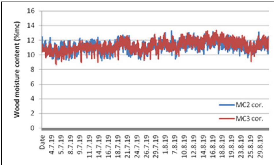
*Fig 141: July/August 2019 temperature corrected equilibrium moisture contents remained low (MC1 provided spurious readings and is not included)*
