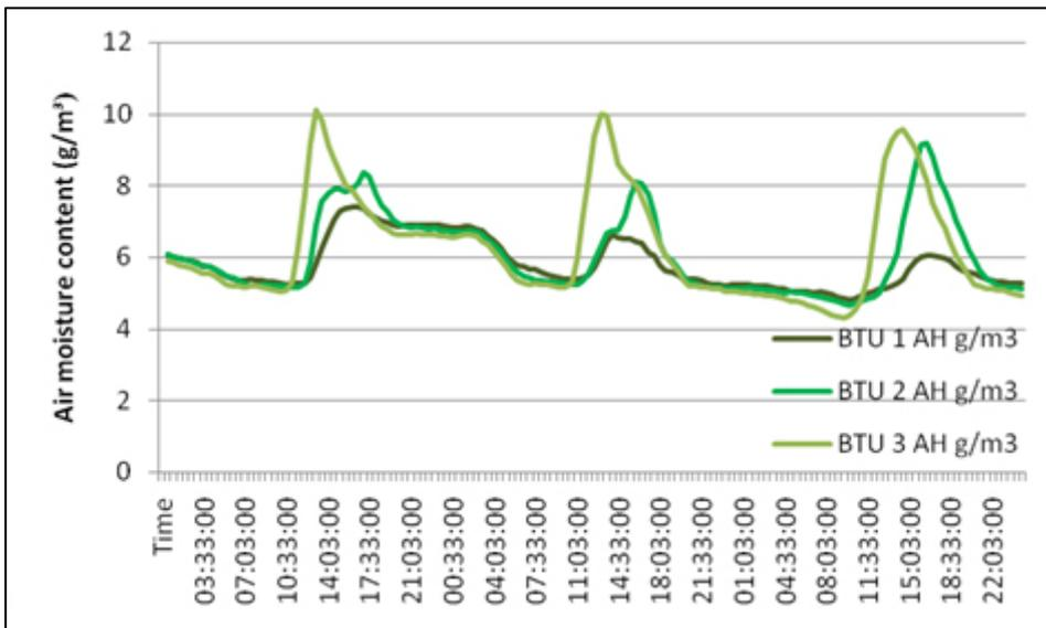
Fig 14: Afternoon spikes in air moisture content ( $\text{g}/\text{m}^3$ ) under tiles, from Figure 12 data
