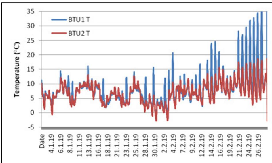
Fig 118: A comparison of January/February 2019 daytime solar gain between the south slope (BTU1) and the north slope (BTU2)
