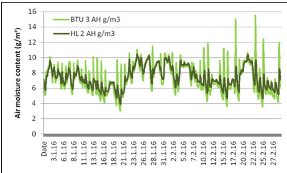
Fig 15: A comparison between air moisture content ( $\text{g/m}^3$ ) at high level (HL) and between tile and underlay (BTU) in the south corner during January and February 2016
