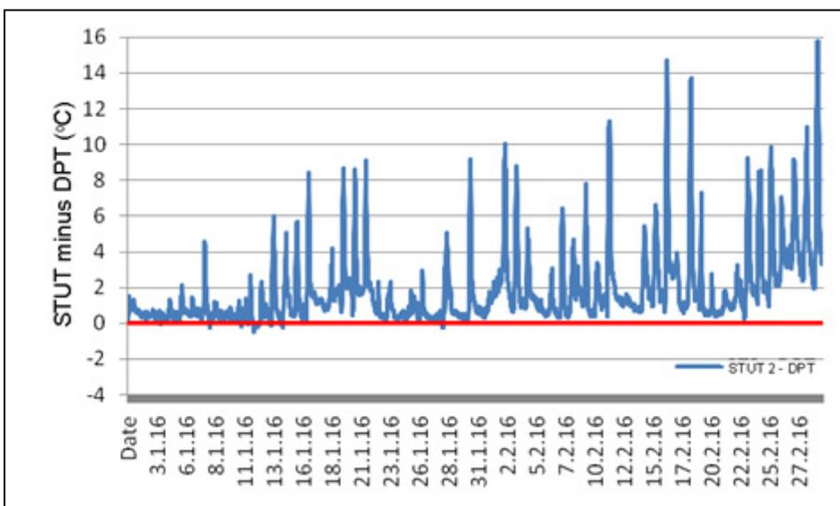
Fig 85: Condensation risk (below red line) on the south slope for January/February 2016 obtained by subtracting dew point (DPT) from surface temperature under tiles (STUT). There was 100mm of insulation between the joists
