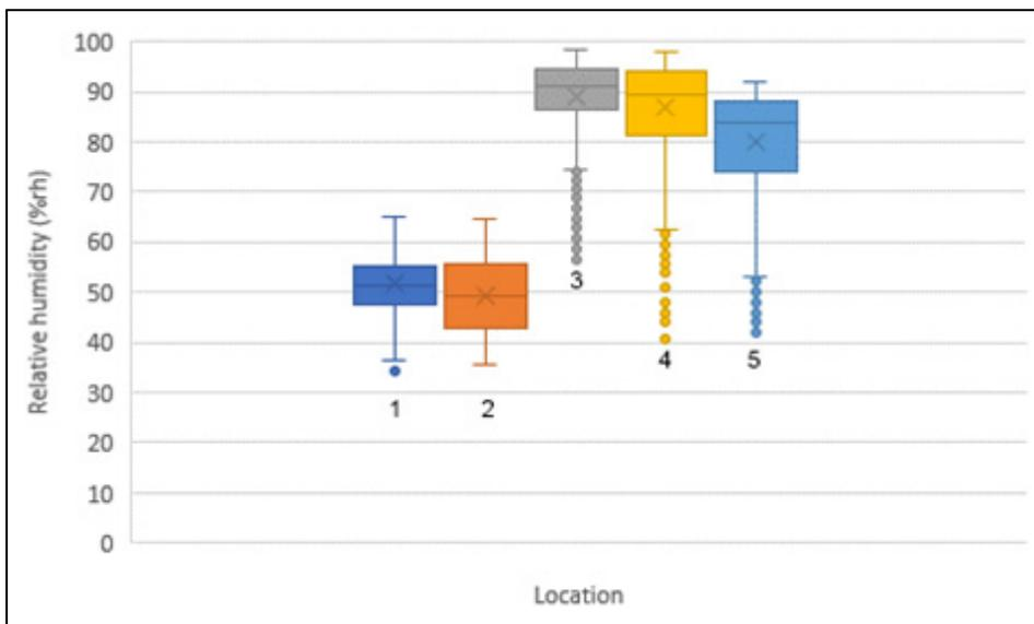
Fig 96: Interquartile relative humidity ranges (%) from below the ceiling (BC) to the exterior for January/February 2016, when there was 100mm of glass fibre insulation
