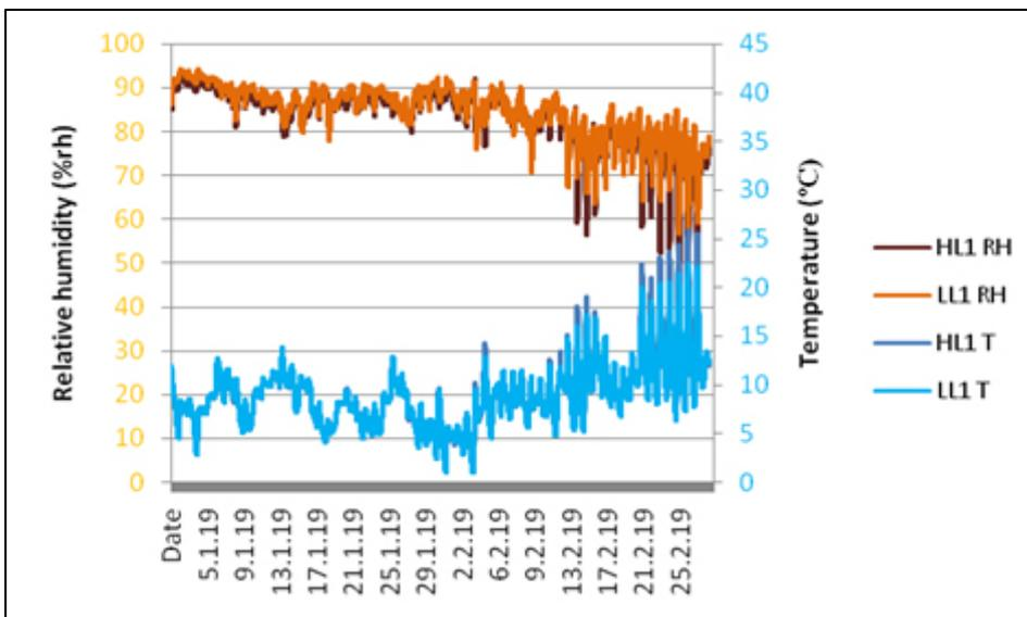
Fig 116: January/February 2019 temperature (°C) and relative humidity (%) comparisons between high (HL) and low level (LL) within the roof space
