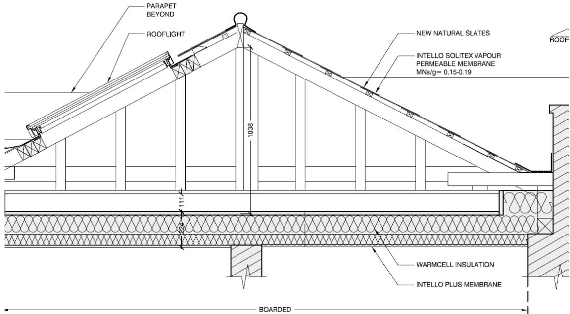
Fig 49: Cross section through attic (Roof 1) (copyright Arboreal Architecture)
