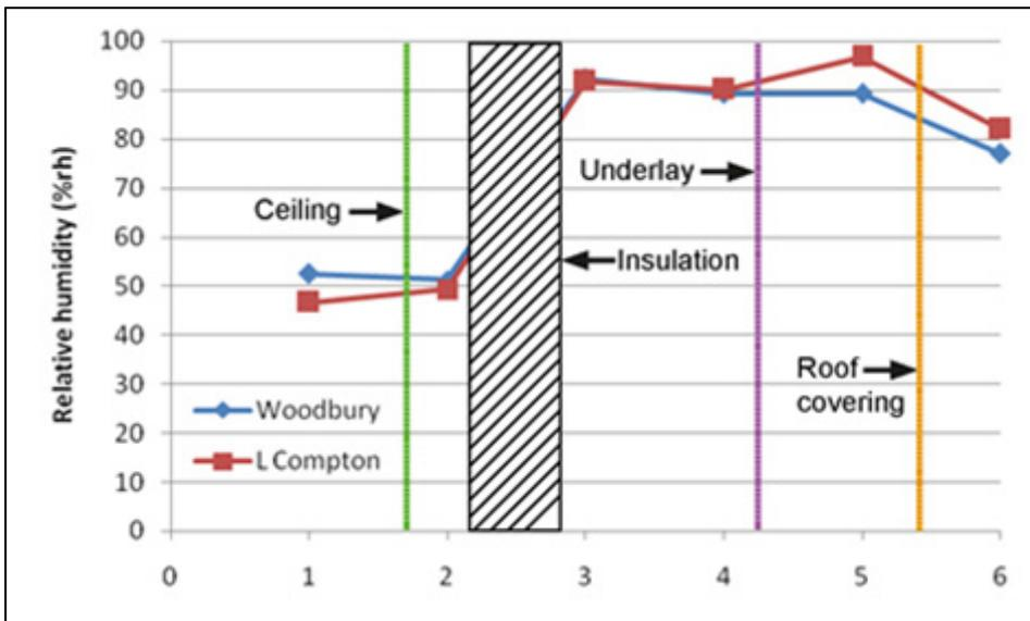
Fig 148: The average relative humidity gradients across the roof from the room (1) to the exterior (6) during the first week of January 2018 ('Woodbury') and the first week of January 2019 ('Long Compton'). 'Woodbury' does not have an underlay
