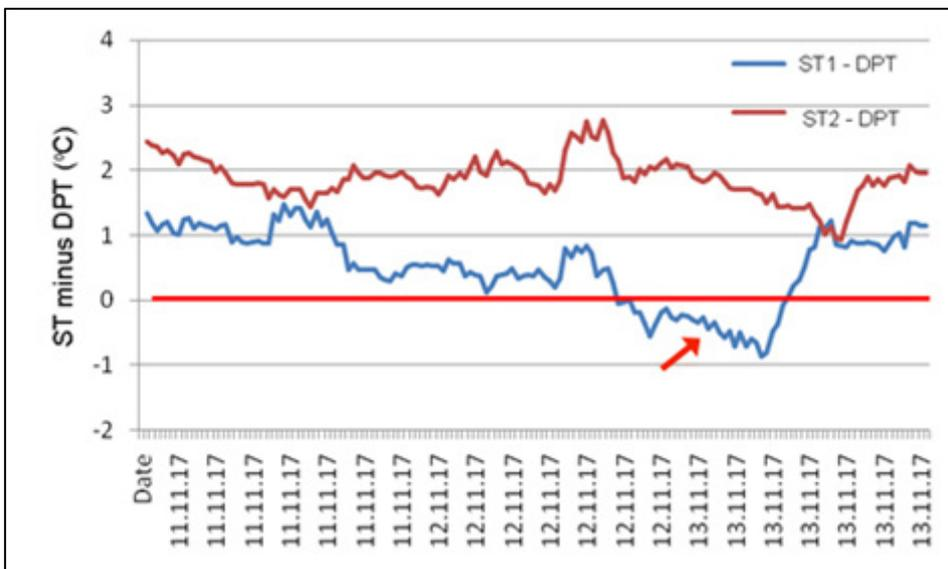
Fig 124: A severe condensation event (below red line) commenced on the night of 12 November 2017 and was observed on 13 November 2017. This is the event photographed in Figure 113
