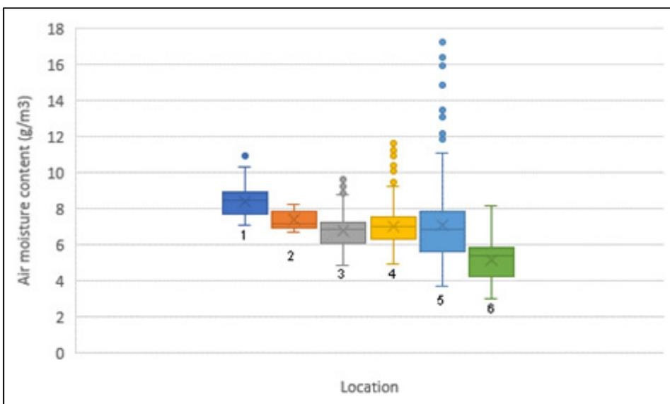
Fig 30: A comparison of median and interquartile range air moisture contents ( $\text{g}/\text{m}^3$ ) from the room (BC1) through the roof space to the exterior for January/February 2016
