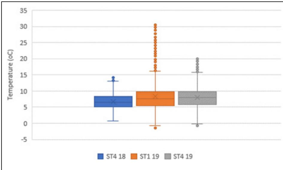
Fig 117: Surface temperature (°C) under felt data for 2018 and 2019
