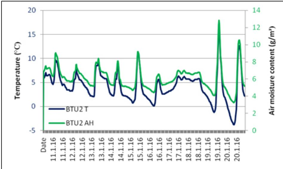
Fig 19: The afternoon spikes in temperature in January 2016 increase the air moisture content
