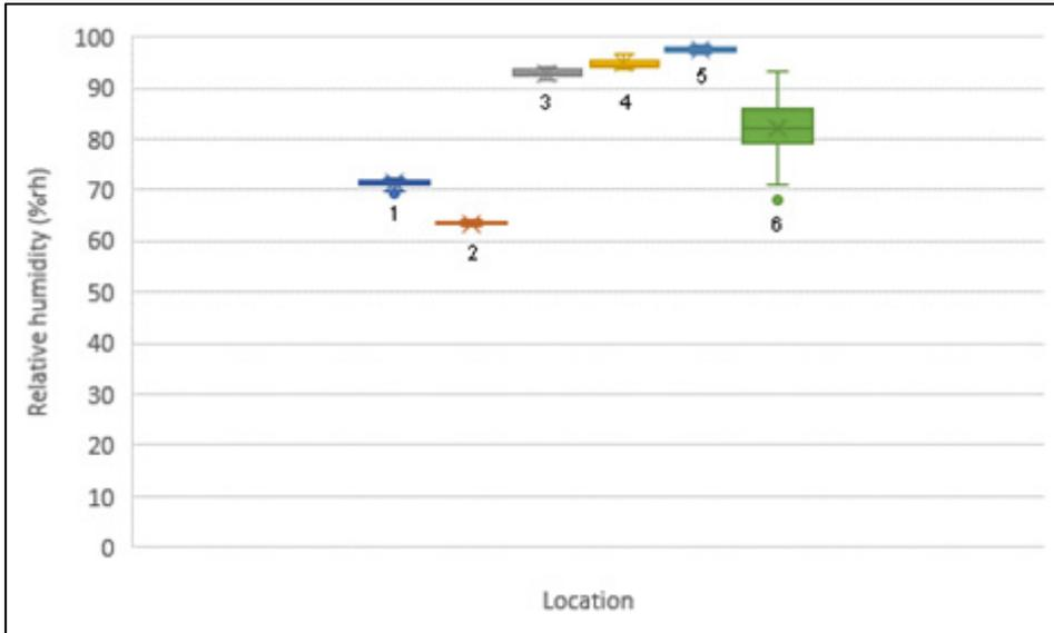
Fig 26: A comparison of median and interquartile range relative humidities (%) from the room (BC1) through the roof space to the exterior for November/December 2015
