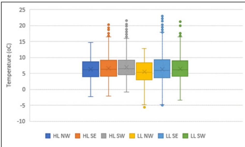
Fig 80: A comparison of high level (HL) and low level (LL) surface temperatures under tiles for January/February 2016
