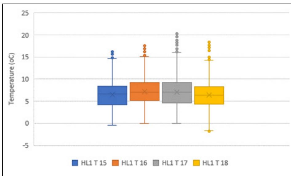
*Fig 90: A comparison of high level (HL) temperatures (January/February) for 2015/16, when there was 100mm of insulation between the joists, and 2017/18, when the thickness had been increased to 300mm*
