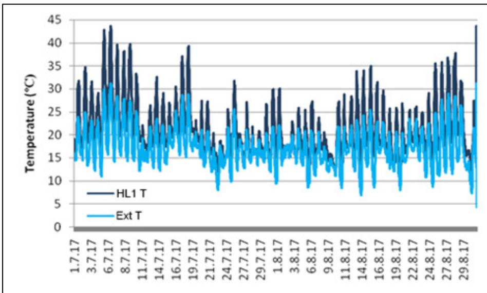
Fig 103: July/August 2017 high level (HL) temperatures compared with exterior (Ext)
