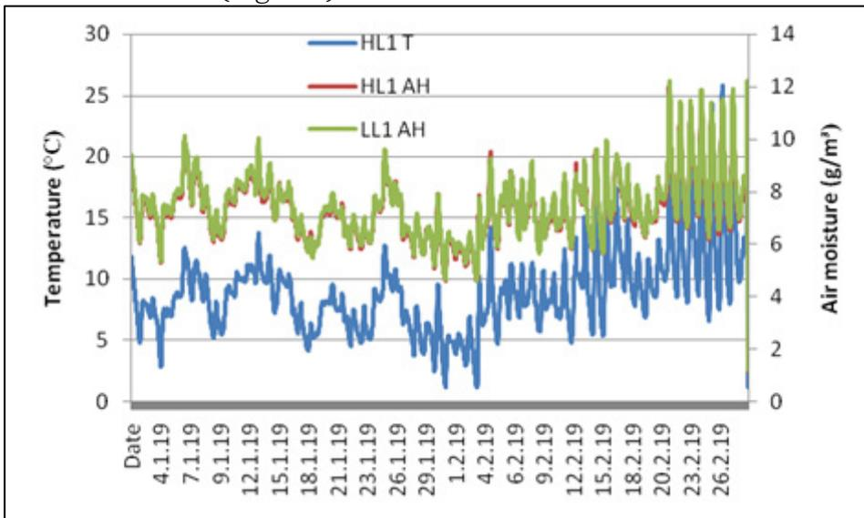
Fig 120: January/February 2019 air moisture contents ( $g/m^3$ ) rise with temperature ( $^{\circ}C$ ) increases, particularly at low level (LL1)
