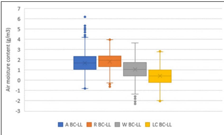
Fig 150: A comparison between the moisture buffering potentials of the four attic floor constructions from 1 January to 23 February 2019. Data obtained by subtracting low level (LL) air moisture content from below ceiling (BC) air moisture content
