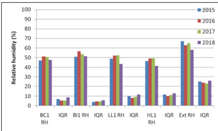
Fig 70: July/August median relative humidity (%) and interquartile ranges (IQR) in the room (BC), below insulation (BI), Roof 1 (HL and LL) and the exterior (Ext) for 2015 to 2018
