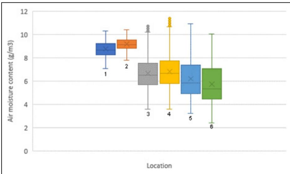
Fig 67: A comparison of median and interquartile range air moisture contents ( $\text{g}/\text{m}^3$ ) from the room (BC1) through the roof space to the exterior for January/February 2016
