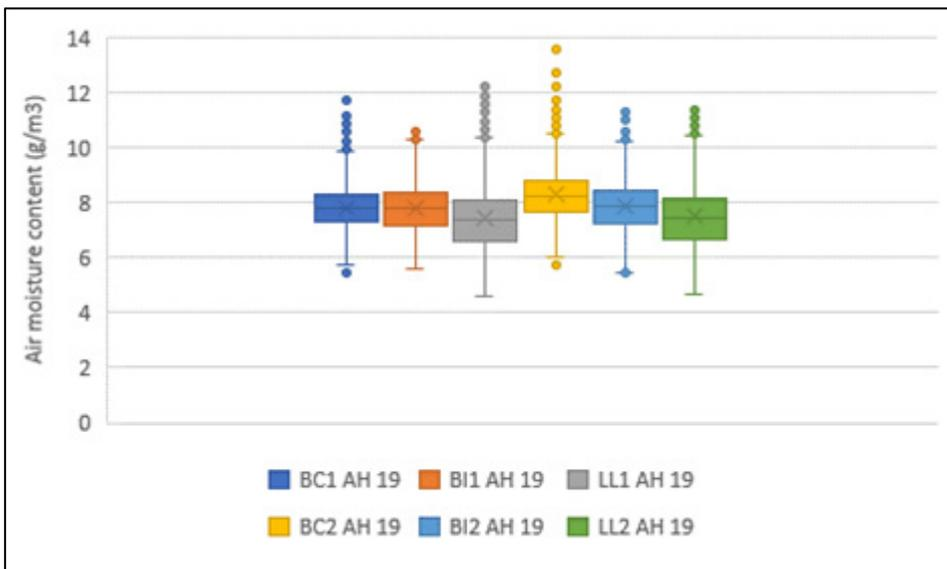
Fig 129: Air moisture content gradients (g/m<sup>3</sup>) from below ceiling (BC) to low level (LL) in the roof for January/February 2019. BC1 is in a spare unused bedroom; BC2 is in the bathroom
