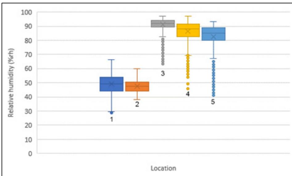
Fig 97: Interquartile relative humidity ranges (%) from below the ceiling (BC) to the exterior for January/February 2017, when there was 300mm of glass fibre insulation
