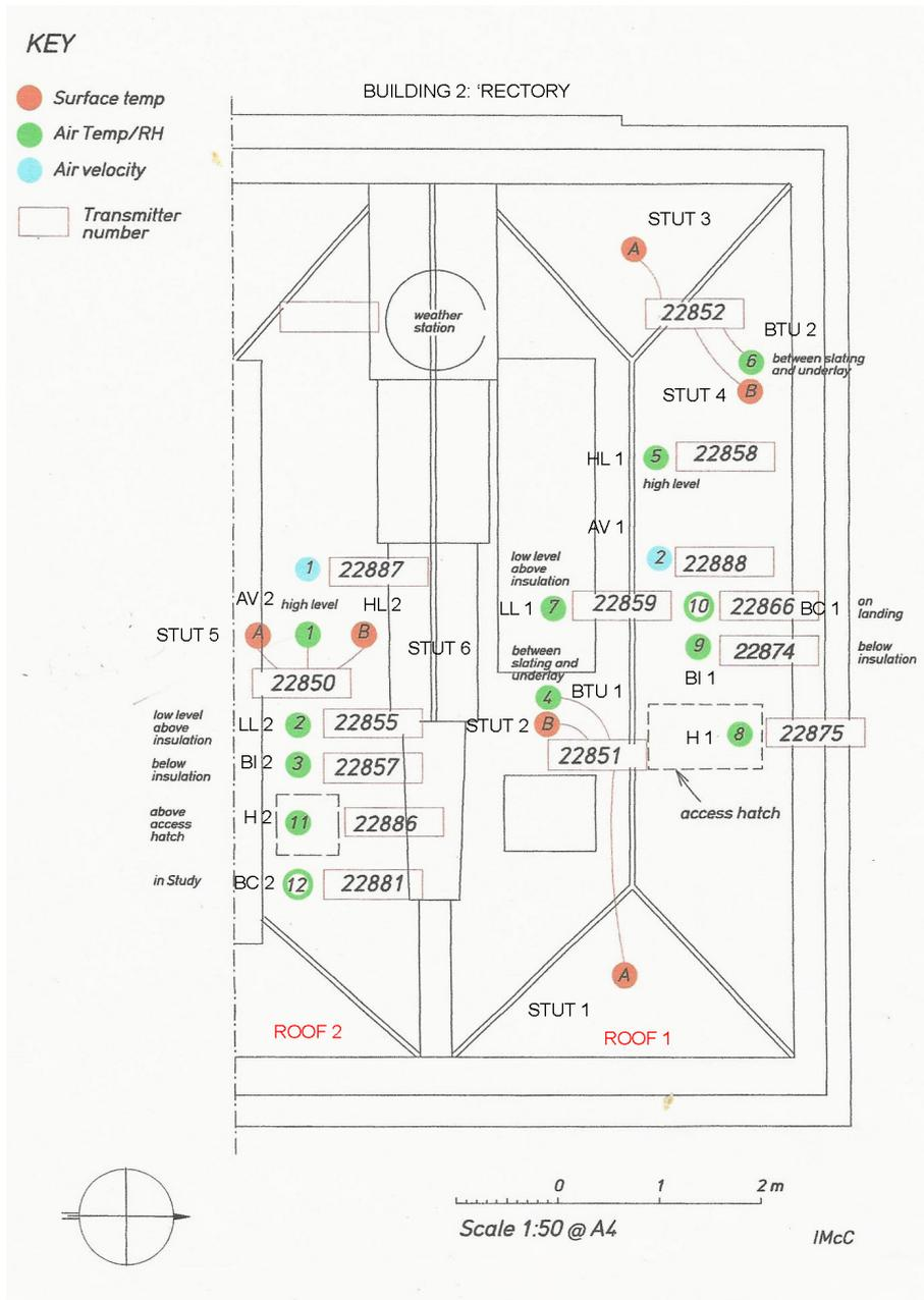
Fig 50: Plan of roof showing sensor positions
