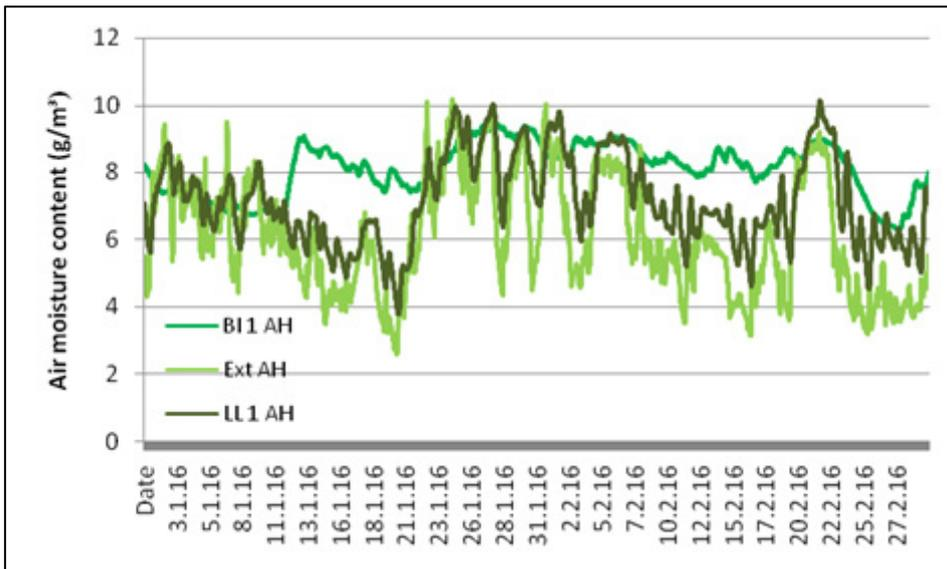
Fig 32: The low level (LL) trace in the roof space is responding to exterior (Ext) air moisture fluctuations, but the below insulation (BI) trace is responding differently
