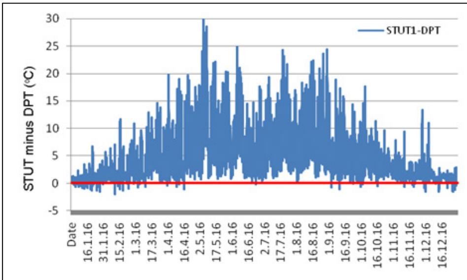
*Fig 109: Condensation risk (below red line) for 2016 obtained by subtracting dew point (DPT) from surface temperature (STUT). This demonstrates the risk of condensation or moisture absorption during the winter months*
