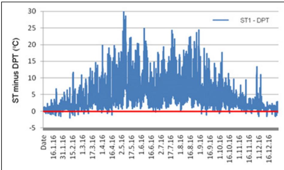
Fig 136: Condensation risk (below red line) for 2016, obtained by subtracting dew point temperature (DPT) from surface temperature under felt (ST1), showing seasonal trends
