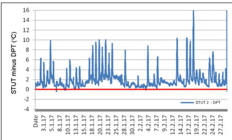
Fig 87: Condensation risk (below red line) on the south slope for January/February 2017 obtained by subtracting dew point (DPT) from surface temperature under tiles (STUT). The thickness of insulation was 300mm
