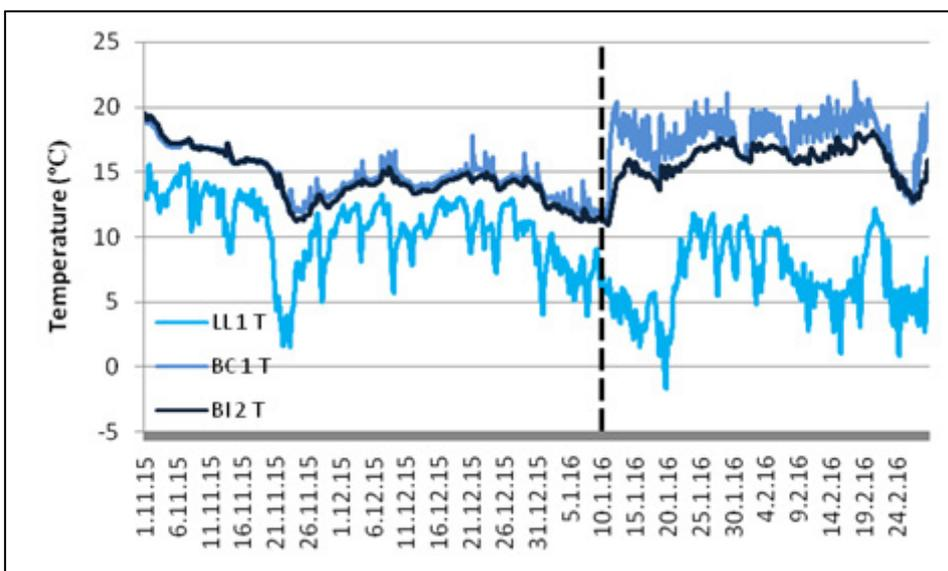
Fig 22: Occupancy (dotted line) and its effects on temperature (°C) below the ceiling (BC), below the insulation (BI) and at low level (LL) within the roof
