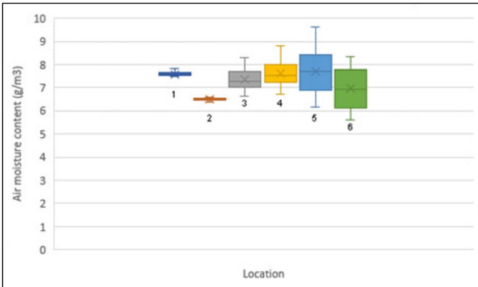
Fig 29: A comparison of median and interquartile range air moisture contents ( $\text{g}/\text{m}^3$ ) from the room (BC1) through the roof space to the exterior for November/December 2015
