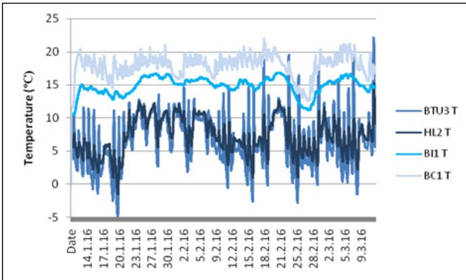
Fig 34: January/February within roof – below the insulation (BI), high level (HL), between tiles and underlay (BTU) – and below ceiling (BC) temperature comparisons for 2016
