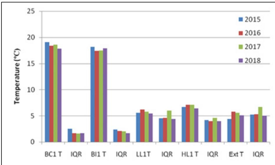
Fig 92: January/February median temperatures (°C) and their interquartile ranges (IQR) in the room (BC), below insulation (BI), low level (LL), high level (HL) and the exterior (Ext) for 2015 to 2018
