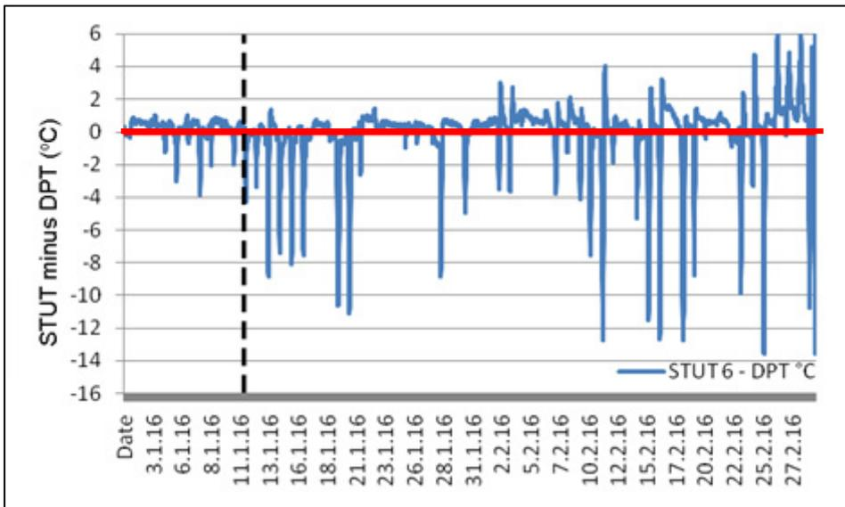
Fig 11: Condensation risk (under red line) in south corner of roof January/February 2016 obtained by subtracting dew point temperature (DPT) from surface temperatures under tiles (STUT). The dotted line is the date occupancy commenced
