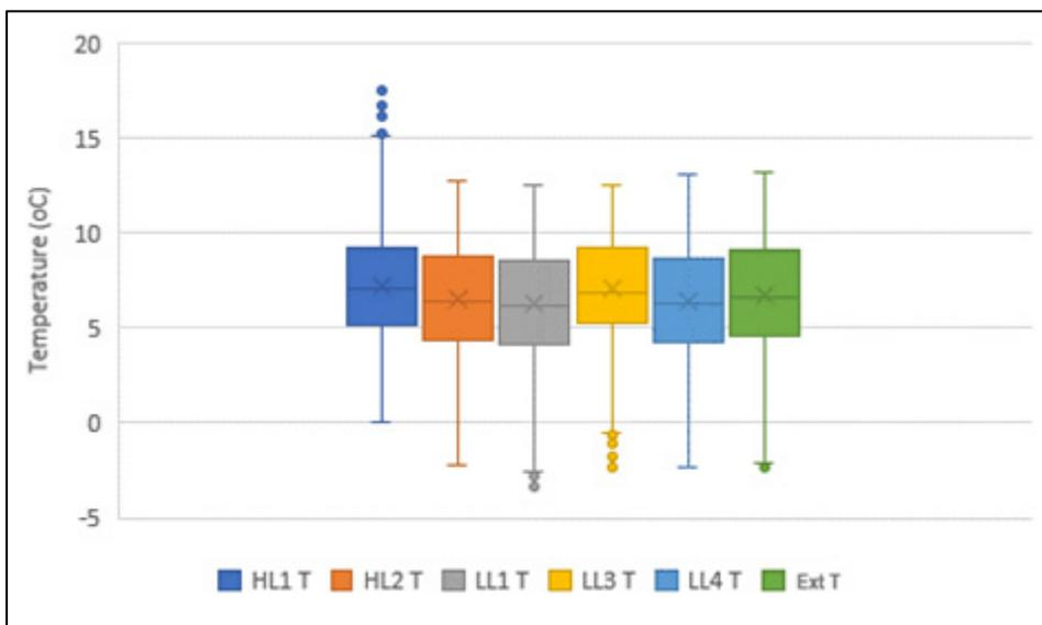
Fig 77: A comparison of median temperatures (°C) and interquartile ranges at high (HL) and low (LL) levels and the exterior (Ext) for January/February 2016
