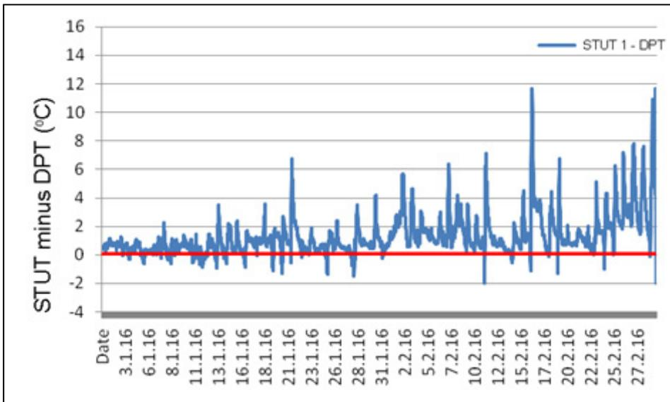
Fig 84: Condensation risk (below red line) on the north slope for January/February 2016 obtained by subtracting dew point (DPT) from surface temperature under tiles (STUT). There was 100mm of insulation between the joists
