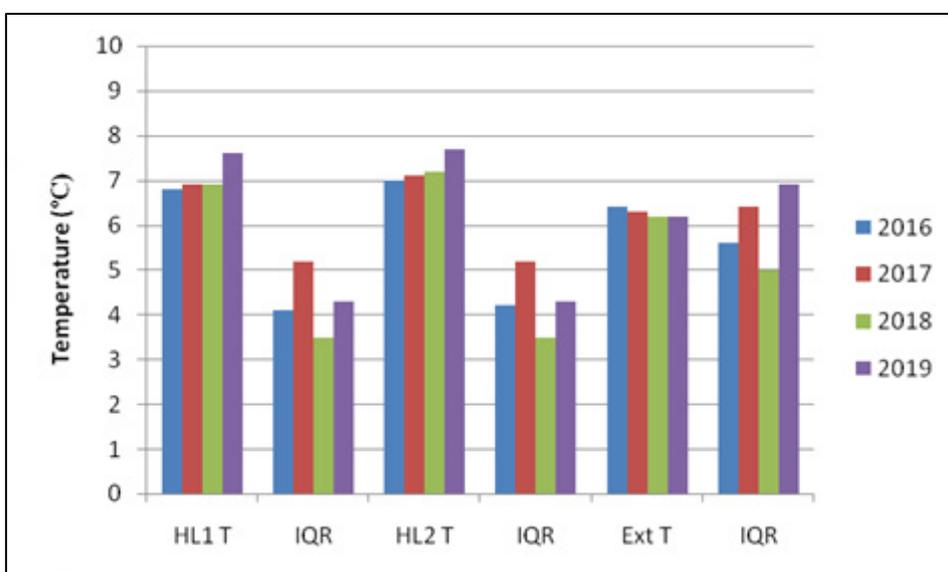
Fig 6: A comparison between high level (HL) and exterior (Ext) median temperatures (°C) and their interquartile ranges (IQR) for January/February 2016 to 2019
