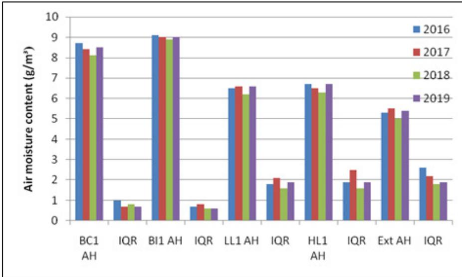
Fig 66: January/February air moisture ( $\text{g}/\text{m}^3$ ) medians and interquartile ranges (IQR) in the room (BC), below insulation (BI), Roofs 1 and 2 (HL and LL) and the exterior (Ext) for 2016 to 2019
