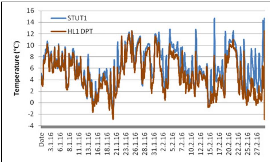
Fig 81: A comparison between high level dew point (HL1 DPT) and surface temperature under the tiles (STUT1)
