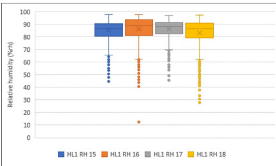
Fig 91: A comparison of high level (HL) relative humidities (January/February) for 2015/16, when there was 100mm of insulation between the joists, and 2017/18, when the thickness had been increased to 300mm
