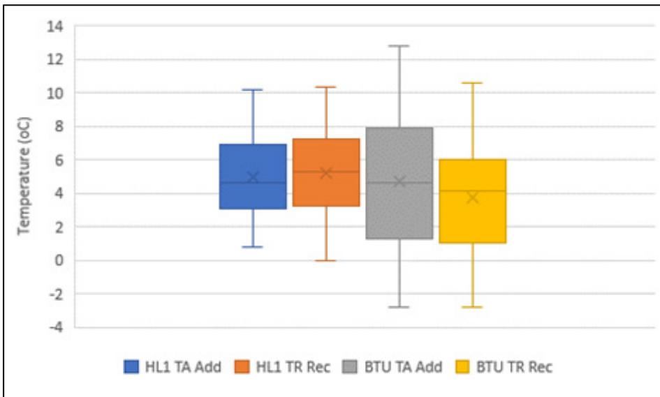
Fig 145: Box plot for high level (HL) and between tile and underlay (BTU) air temperatures for the first seven days of January 2017 at 'Addison' (A) and 'Rectory' (R)
