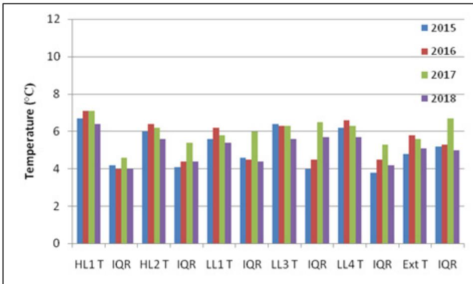
Fig 76: January/February median temperatures (°C) and interquartile ranges (IQR) at different levels and orientations for high level (HL), low level (LL) and exterior (Ext)
