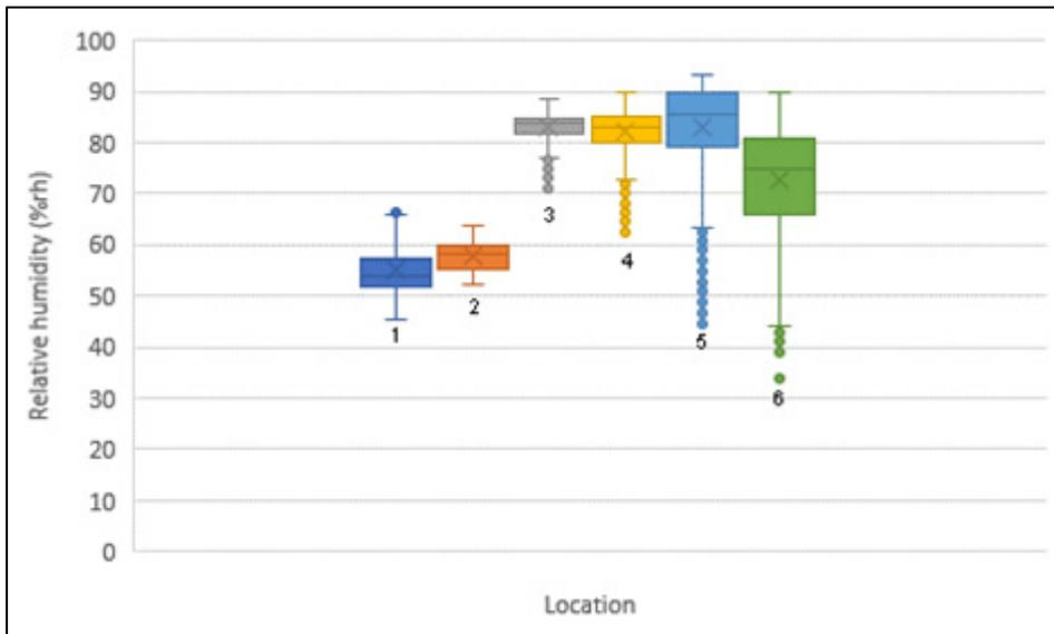
Fig 65: A comparison of median and interquartile range relative humidities (%) from the room (BC1) through the roof space to the exterior for January/February 2016
