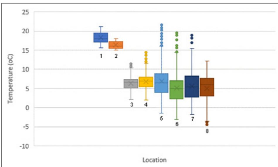
Fig 24: A comparison of median and interquartile range temperatures from the room (BC1) through the roof space to the exterior from 11 January to 29 February 2016
