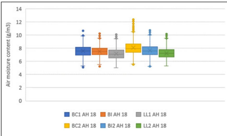
Fig 127: Air moisture content gradients (g/m³) from below ceiling (BC) to low level (LL) in the roof for January/February 2018. BC1 is in a spare unused bedroom; BC2 is in the bathroom
