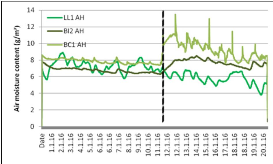
Fig 31: Occupancy (dotted line) and its effects on air moisture contents ( $\text{g}/\text{m}^3$ ) below the ceiling (BC), below the insulation (BI) and at low level (LL) within the roof
