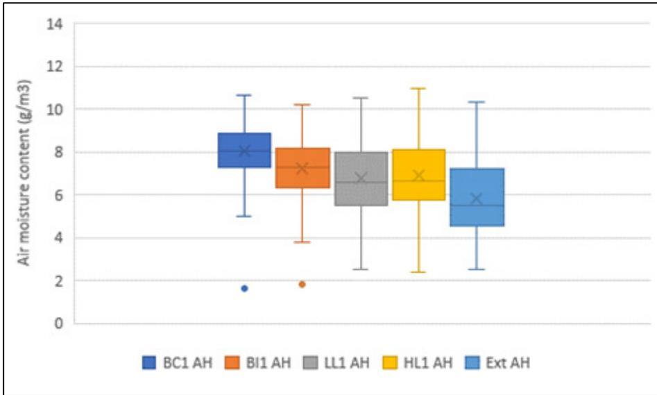
Fig 98: Interquartile air moisture content ( $\text{g}/\text{m}^3$ ) ranges from below the ceiling (BC) to the exterior (Ext) for January/February 2016, when there was 100mm of glass fibre insulation
