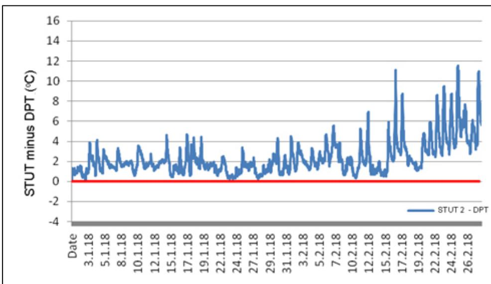
Fig 89: Condensation risk (below red line) on the south slope for January/February 2018 obtained by subtracting dew point (DPT) from surface temperature under tiles (STUT). The thickness of insulation was 300mm
