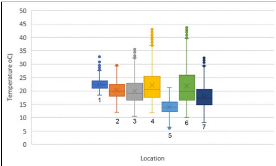
Fig 106: Median and interquartile temperatures (°C) for July/August 2016 from the room, through the roof space to the exterior
