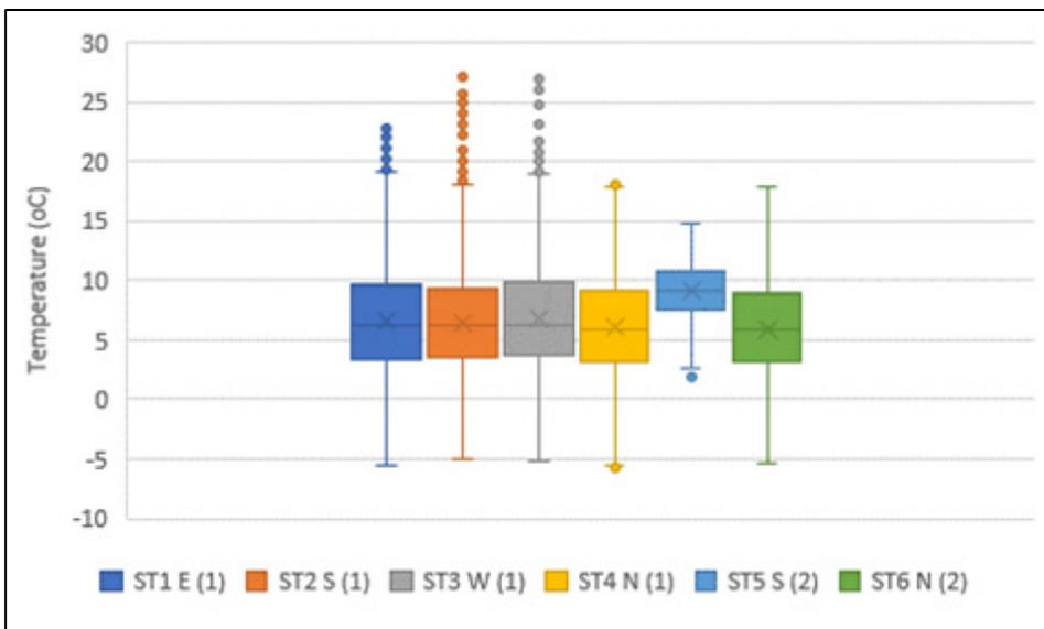
Fig 57: Box plot of surface temperature under slate (°C) for January/February 2016
