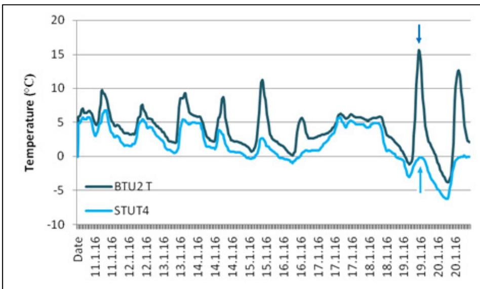
Fig 20: The arrows show that the underside (STUT = light blue trace) does not reach the same temperature as the air (BTU = dark trace)
