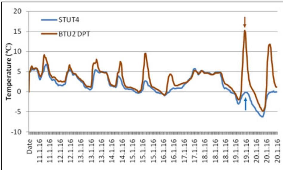
Fig 21: The afternoon spikes in temperature increase the air moisture content and, therefore, the dew point, particularly on the afternoon of 19 January 2016 (arrows)
