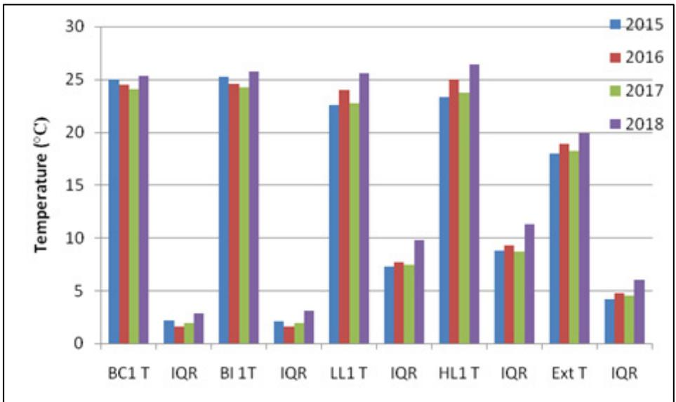
Fig 68: January/February median temperatures (°C) and their interquartile ranges (IQR) in the room (BC), below insulation (BI), Roof 1 (HL and LL) and the exterior (Ext) for 2016 to 2019
