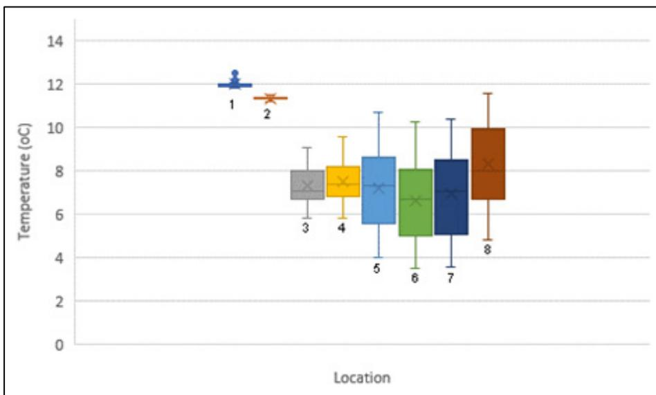
Fig 23: A comparison of median and interquartile range temperatures from the room (BC1) through the roof space to the exterior from 11 November 2015 to 10 January 2016
