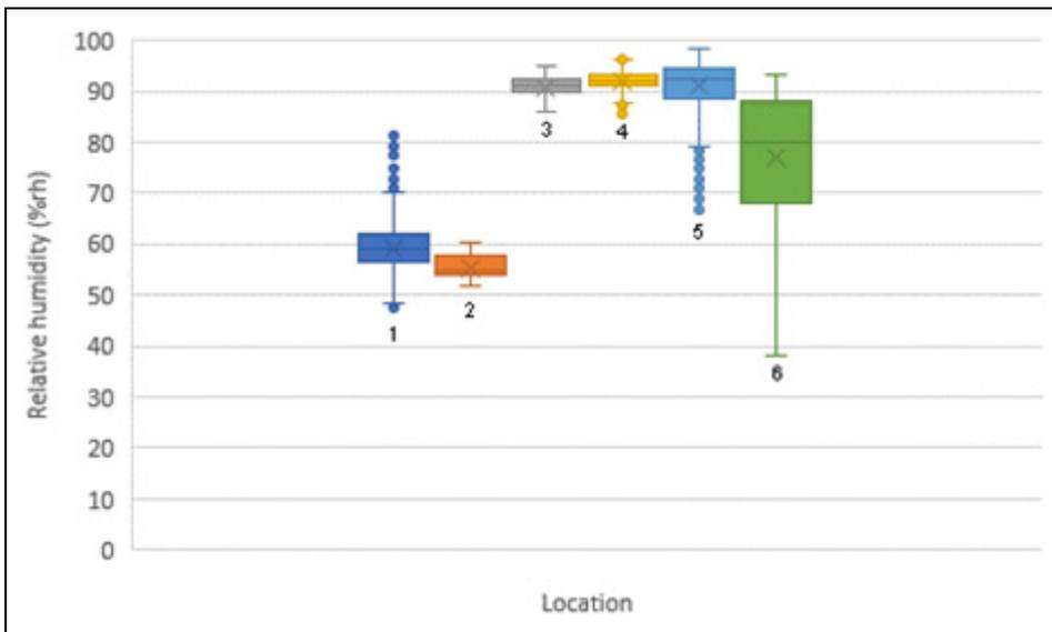
Fig 27: A comparison of median and interquartile range relative humidities (%) from the room (BC1) through the roof space to the exterior for January/February 2016
