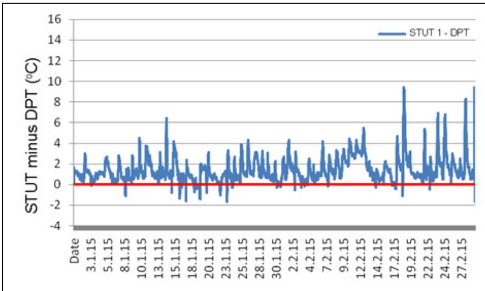
Fig 82: Condensation risk (below red line) on the north slope for January/February 2015 obtained by subtracting dew point (DPT) from surface temperature under tiles (STUT). There was 100mm of insulation between the joists
