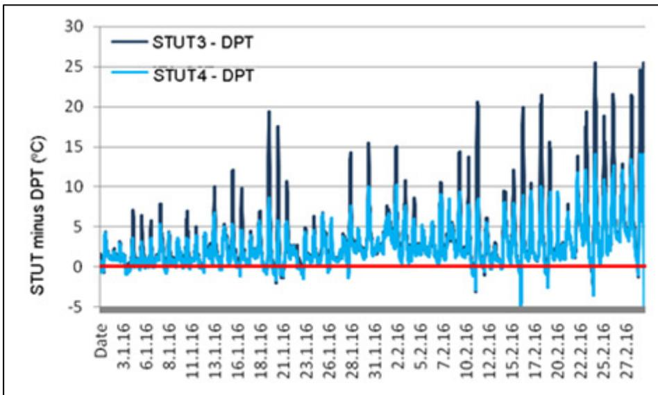
Fig 59: Condensation risk (below red line) for January/February 2016 obtained by subtracting dew point temperature (DPT) from surface temperatures 3 and 4 (west and north) under slates (STUT)
