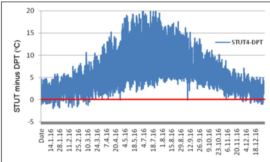
Fig 73: The condensation risk (below red line) on the north slope of the roof during 2016, obtained by subtracting dew point (DPT) from surface temperature under slates (STUT)
