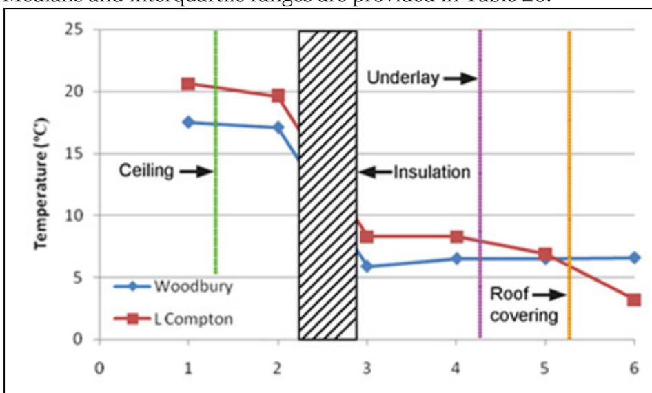
Fig 147: The average temperature gradients across the roof from the room (1) to the exterior (6) during the first week of January 2018 (‘Woodbury’) and the first week of January 2019 (‘Long Compton’). ‘Woodbury’ does not have an underlay
