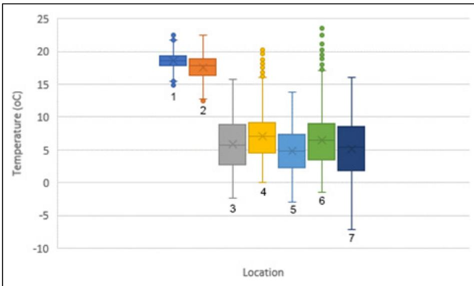
Fig 95: Interquartile temperature ranges (°C) from below the ceiling (BC) to the exterior for January/February 2017, when there was 300mm of glass fibre insulation
