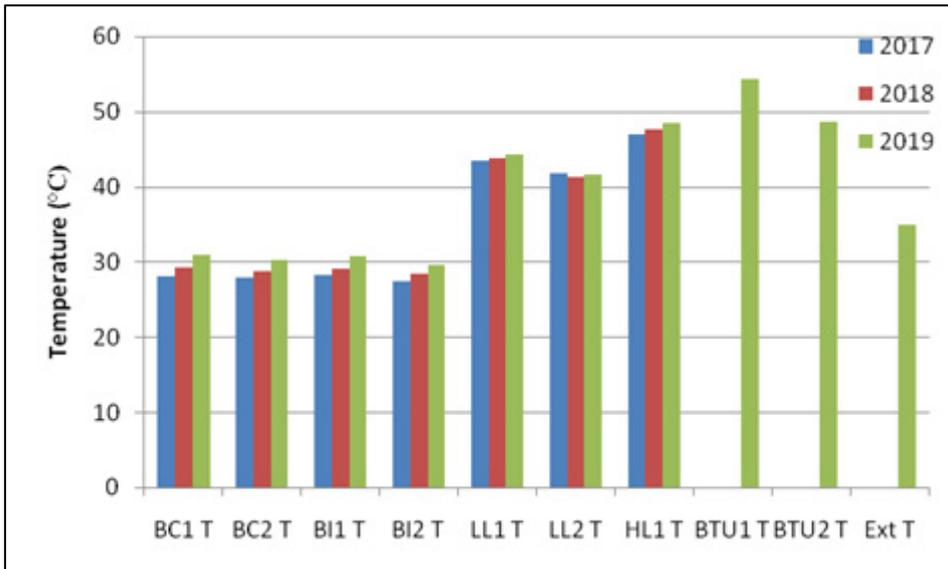
Fig 133: July/August maximum temperatures (°C) recorded in the rooms (BC), beneath insulation (BI), low level (LL), high level (HL), between tiles and underlay (BTU) and exterior (Ext) during 2017 to 2019. LL1 and BTU1 are on the south side; LL2 and BTU2 are on the north side; HL1 is below the ridge
