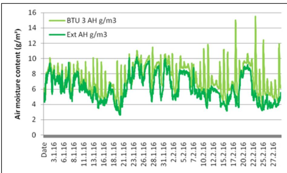
Fig 12: Air moisture content ( $g/m^3$ ) between tiles and underlay (BTU) compared with exterior (Ext) during January and February 2016
