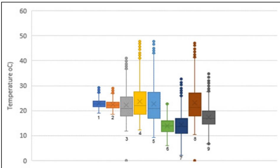
Fig 134: Median and interquartile temperatures (°C) for July/August 2019 from the room, through the roof space to the exterior
