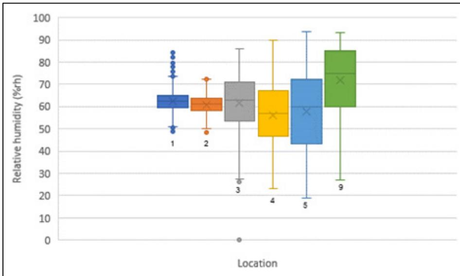
Fig 135: Median and interquartile relative humidities (°C) for July/August 2019 from the room, through the roof space to the exterior
