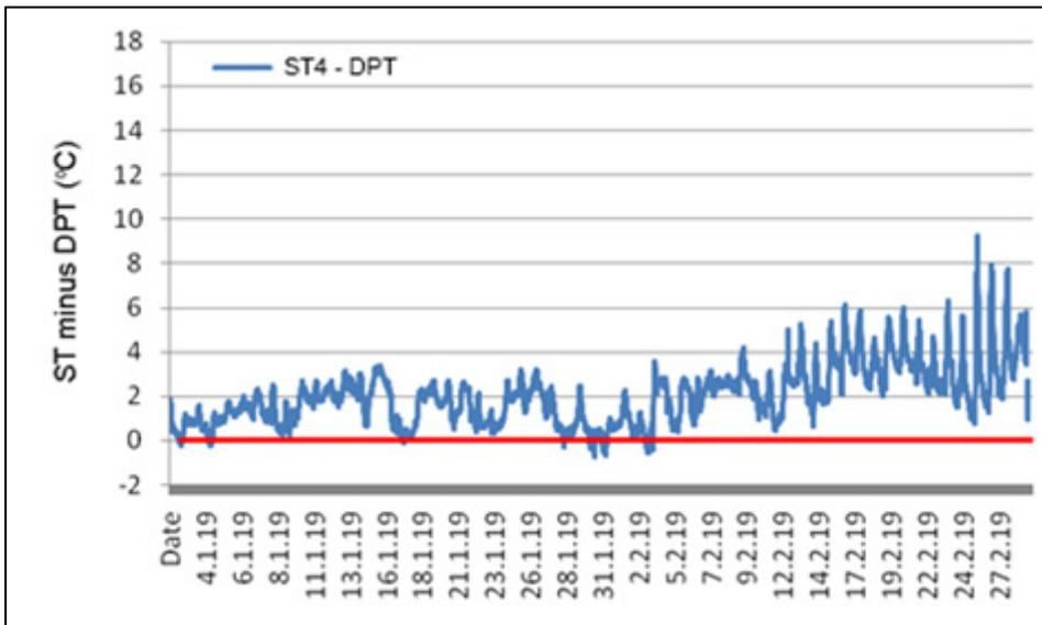
Fig 123: January/February 2019 condensation risk (under red line) for the north slope of the roof
