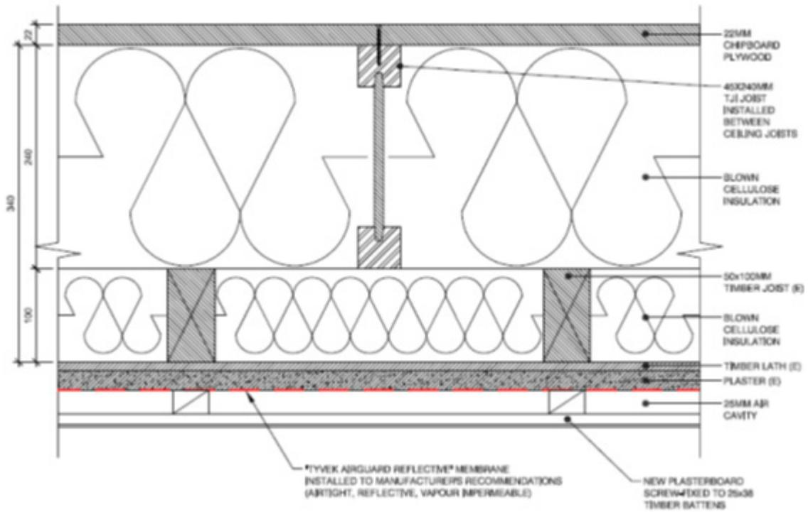
Fig 2: Attic floor construction (copyright Arboreal Architecture)
