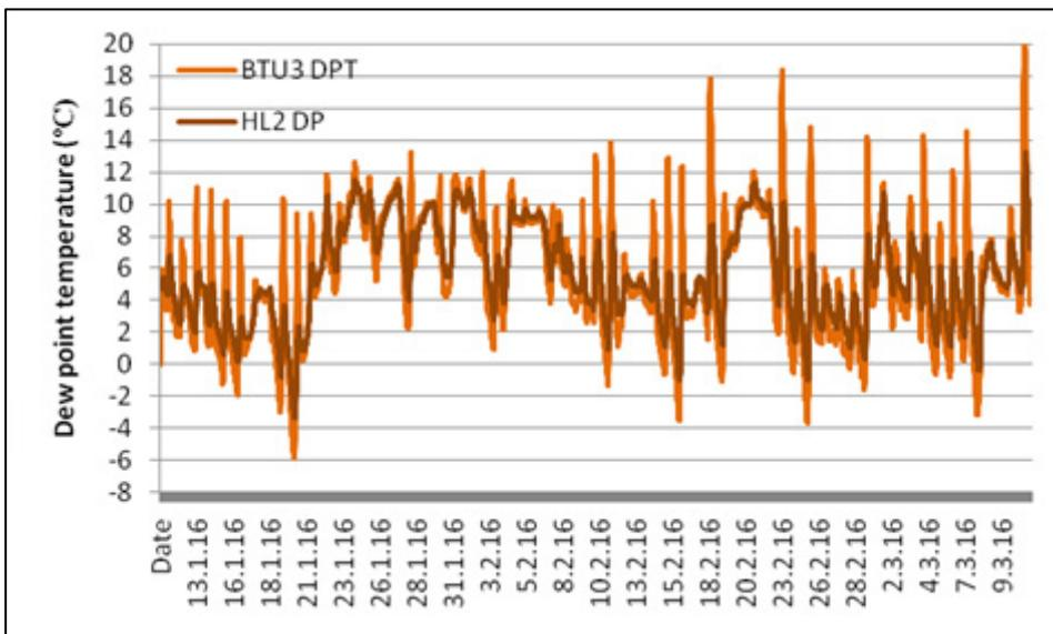
Fig 16: A comparison between dew point temperatures ( $^{\circ}\text{C}$ ) at high level (HL) and between tile and underlay (BTU) in the south corner during January and February 2016
