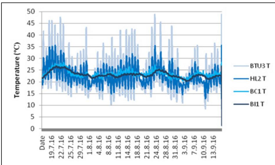
Fig 35: July/August within roof – below the insulation (BI), high level (HL), between tiles and underlay (BTU) – and below ceiling (BC) temperature comparisons for 2016
