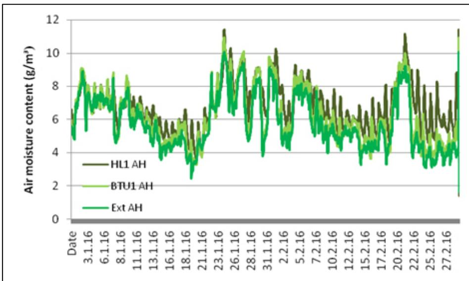
Fig 61: Air moisture content ( $\text{g}/\text{m}^3$ ) at high level (HL), between slates and underlay (BTU) and exterior (Ext) for January/February 2016
