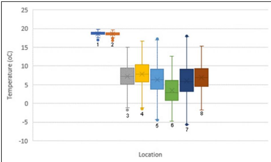
Fig 63: A comparison of median and interquartile range temperatures from the room (BC1) through the roof space to the exterior for January/February 2016
