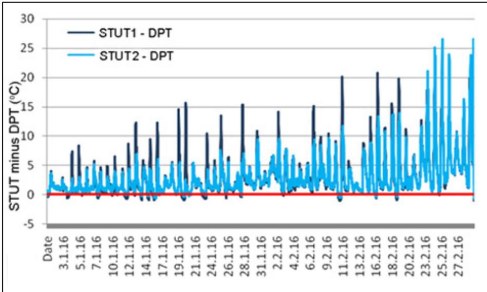
Fig 58: Condensation risk (below red line) for January/February 2016 obtained by subtracting dew point temperature (DPT) from surface temperatures 1 and 2 (east and south) under slates (STUT)
