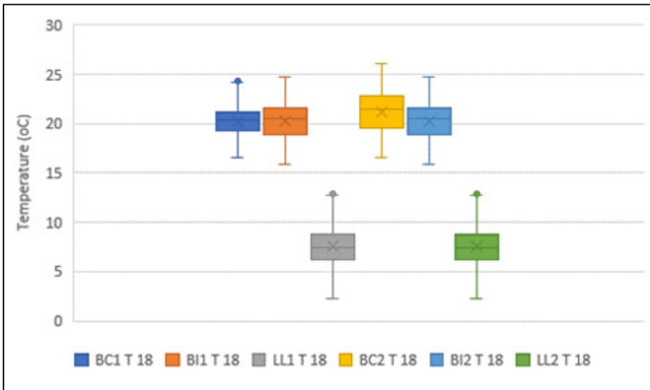
Fig 126: Temperature gradients (°C) from below ceiling (BC) to low level (LL) in the roof for January/February 2018. BC1 is in a spare unused bedroom; BC2 is in the bathroom
