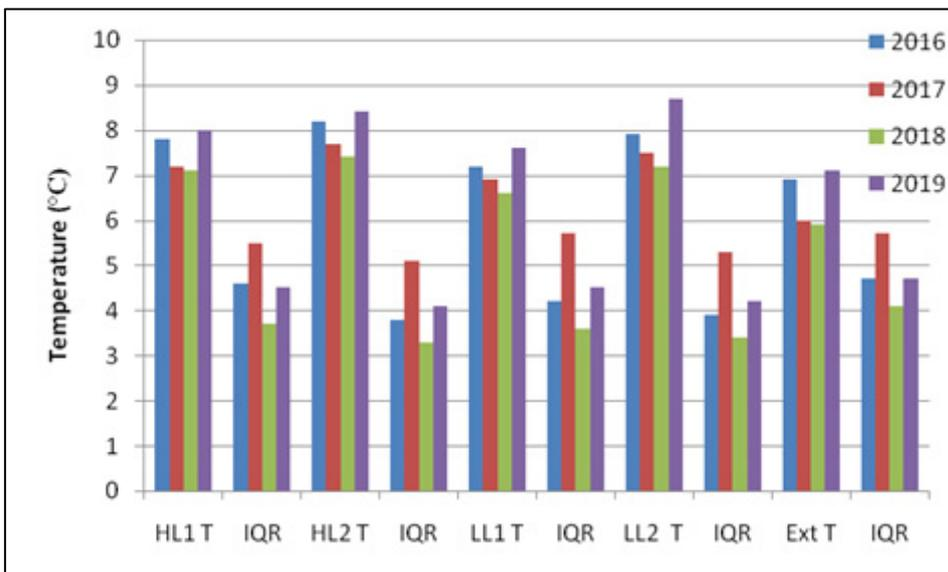
Fig 52: January/February median temperatures (°C) at high (HL) and low (LL) levels, with their interquartile ranges (IQR) compared with exterior (Ext) for 2016 to 2019
