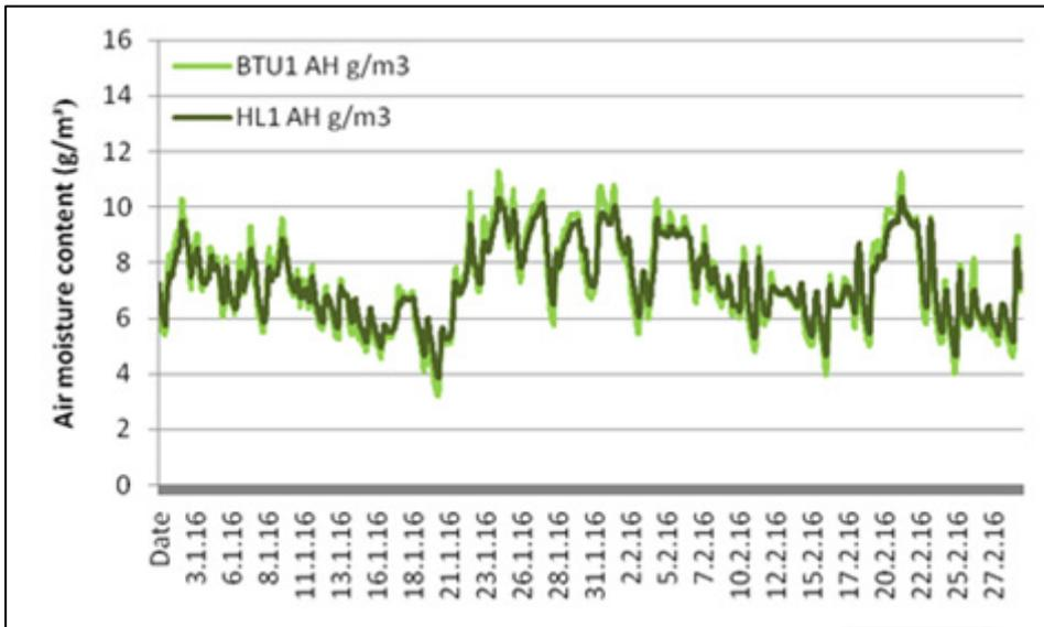
Fig 17: A comparison between air moisture content ( $\text{g}/\text{m}^3$ ) at high level (HL) and between tile and underlay (BTU) in the north corner during January and February 2016
