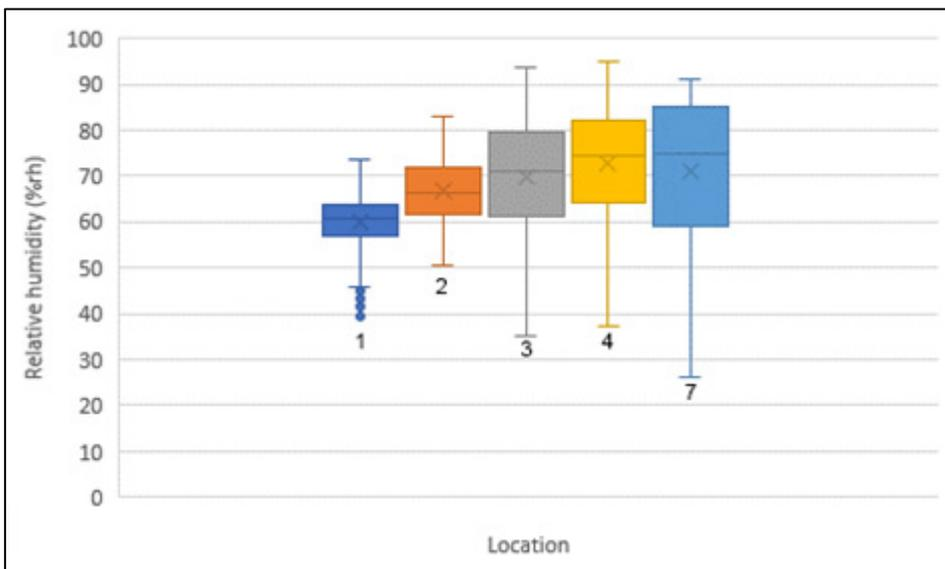
Fig 107: Median and interquartile relative humidities (%) for July/August 2016 from the room, through the roof space to the exterior
