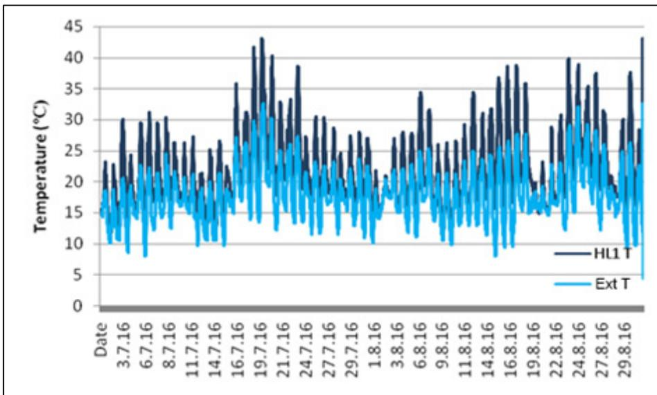
Fig 102: July/August 2016 high level (HL) temperatures compared with exterior (Ext)
