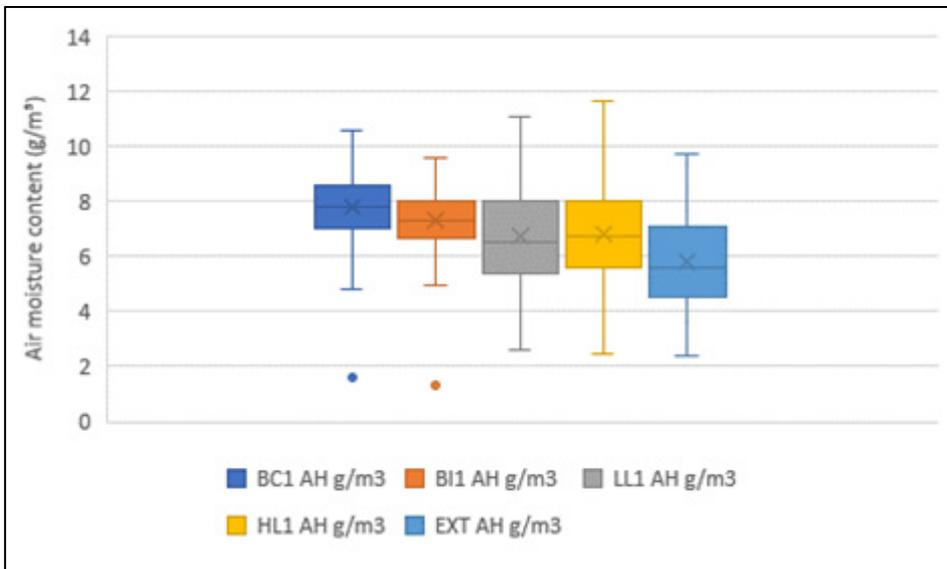
Fig 99: Interquartile air moisture content ( $\text{g}/\text{m}^3$ ) ranges from below the ceiling (BC) to the exterior (Ext) for January/February 2017, when there was 300mm of glass fibre insulation
