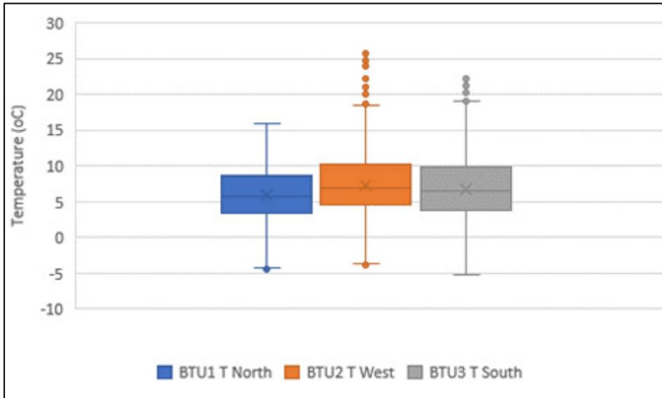
Fig 4: Air temperatures (°C) under the tiles for different roof slope orientations. The upper outliers (dots) are solar gain
