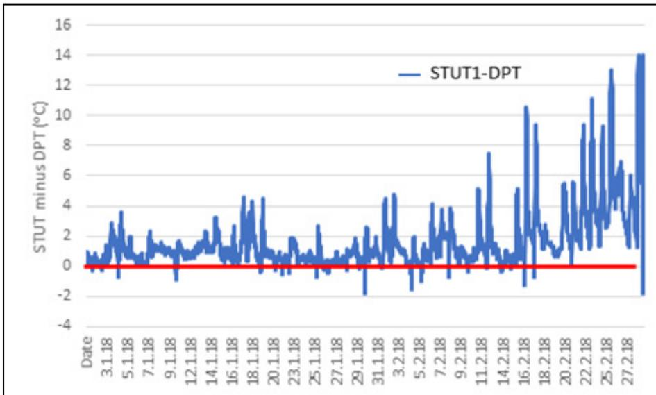
Fig 88: Condensation risk (below red line) on the north slope for January/February 2018 obtained by subtracting dew point (DPT) from surface temperature under tiles (STUT). The thickness of insulation was 300mm
