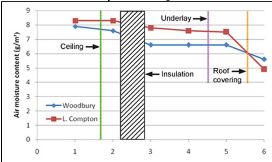
Fig 149: The average air moisture gradients across the roof from the room (1) to the exterior (6) during the first week of January 2018 ('Woodbury') and the first week of January 2019 ('Long Compton'). 'Woodbury' does not have an underlay
