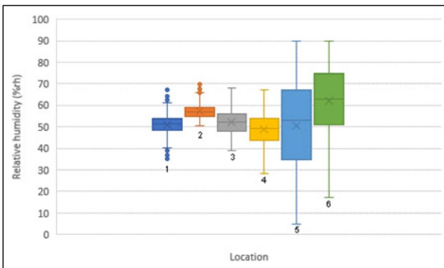
Fig 71: Box plot of relative humidity (%) distribution from the room (BC1) across the roof to the exterior
