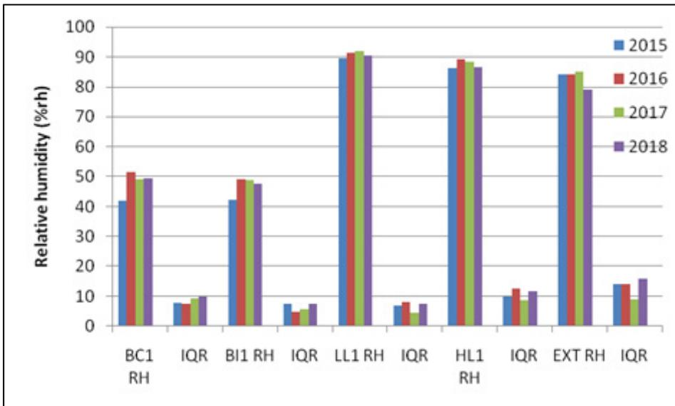
Fig 93: Median relative humidities (%) and their interquartile ranges (IQR) in the room (BC), below insulation (BI), low level (LL), high level (HL) and the exterior (Ext) for 2015 to 2018
