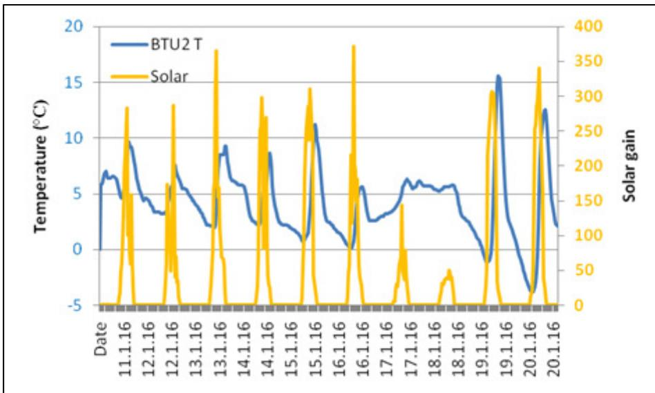
Fig 18: A comparison between afternoon temperature spikes ( $^{\circ}\text{C}$ ) and solar gain (irradiance  $\text{W}/\text{m}^2$ ) in January 2016
