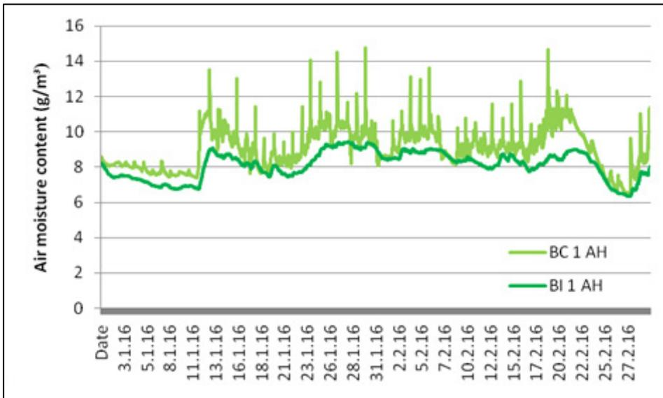
Fig 33: A comparison of the air moisture content ( $\text{g}/\text{m}^3$ ) below the ceiling (BC) and below the insulation (BI). The underlying trace shapes are similar
