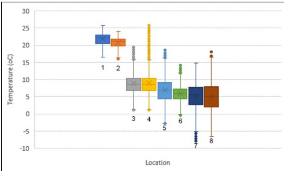
Fig 130: Temperature profile from room to exterior for January/February 2019
