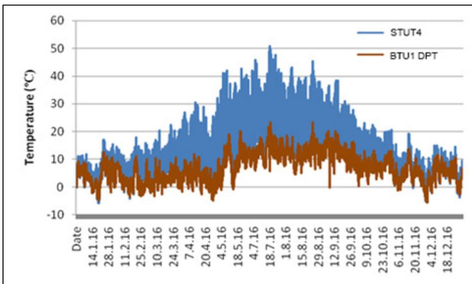
Fig 72: Dew point (DPT) and surface temperature under slates (STUT) for 2016
