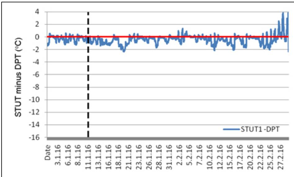
Fig 9: Condensation risk (under red line) in north corner of roof January/February 2016 obtained by subtracting dew point temperature (DPT) from surface temperatures under tiles (STUT). The dotted line is the date occupancy commenced
