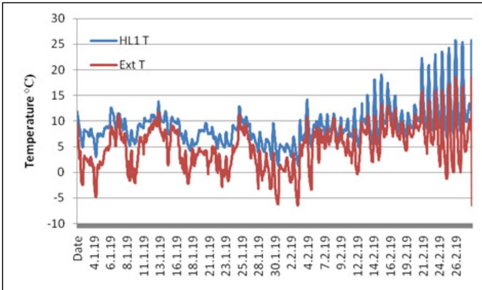
Fig 119: In January/February 2019, the roof environment (HL1) is warmer than the exterior (Ext) because of solar gain
