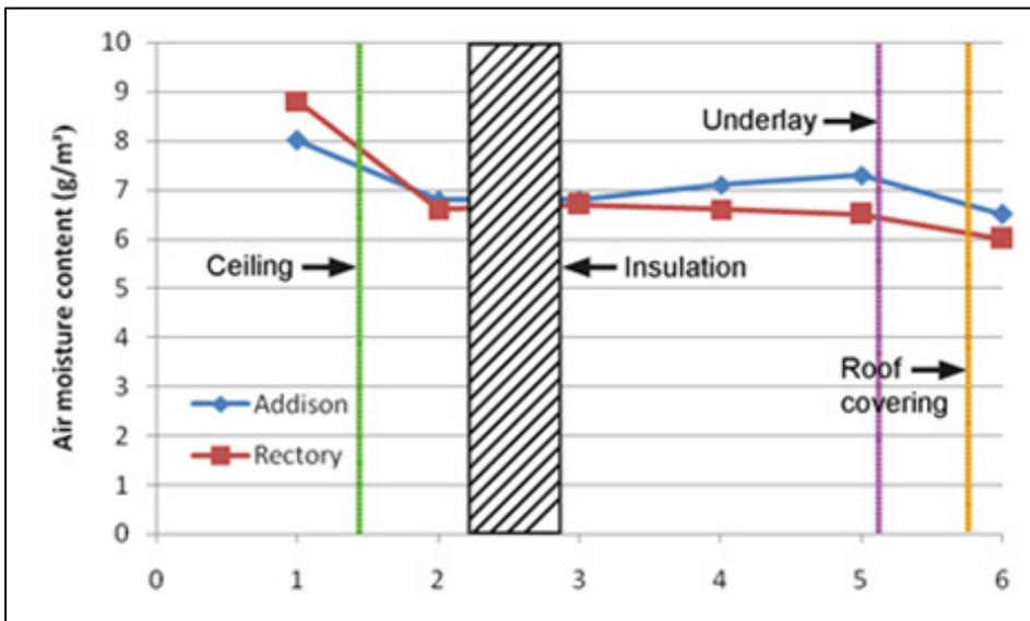
Fig 144: The average air moisture content gradients across the roof from the room (1) to the exterior (6) during the first week of January 2017
