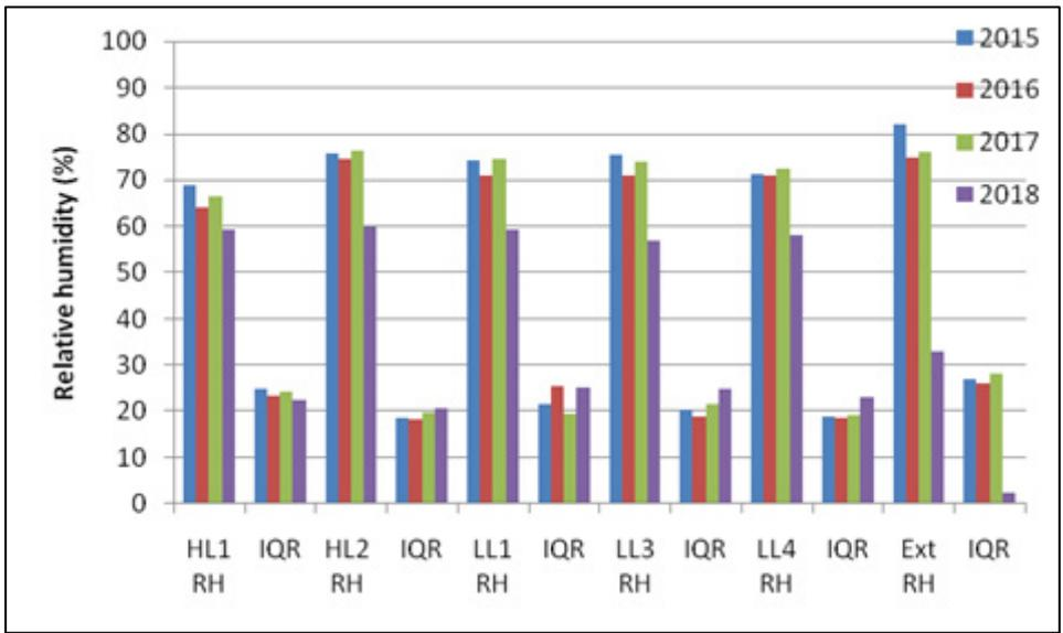
Fig 101: July/August average high level (HL) and low level (LL) relative humidity (%) compared with exterior (Ext) for 2015 to 2018
