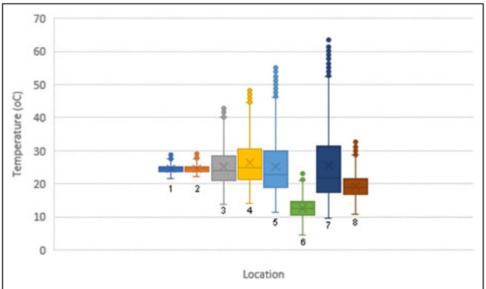
Fig 69: Box plot of temperature distribution from the room (BC1) across the roof to the exterior for 2016
