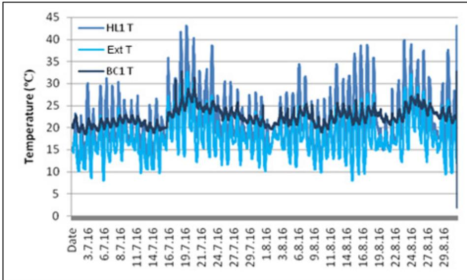
Fig 108: Room (BC1), roof (HL1) and exterior (Ext) temperatures compared for July/August 2016
