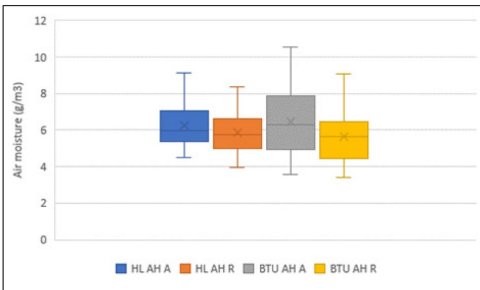
Fig 146: Box plot for high level (HL) and between tile and underlay (BTU) air moisture contents for the first seven days of January 2017 at ‘Addison’ (A) and ‘Rectory’ (R)
