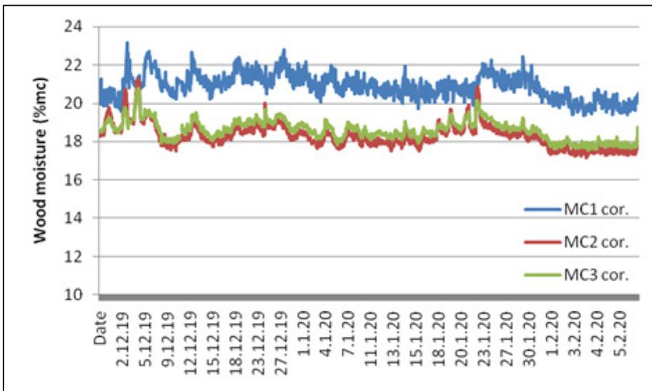
Fig 140: Temperature corrected data from December 2019 to the beginning of February 2020. The underside of the rafter (MC2) and the joist (MC3) have very similar moisture contents, whereas just under the felt (MC1) is much damper
