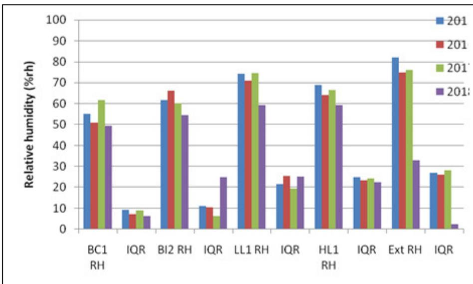
Fig 105: July/August average relative humidities (%) in the room (BC), below insulation (BI), high level (HL), low level (LL) and the exterior (Ext) for 2015 to 2018
