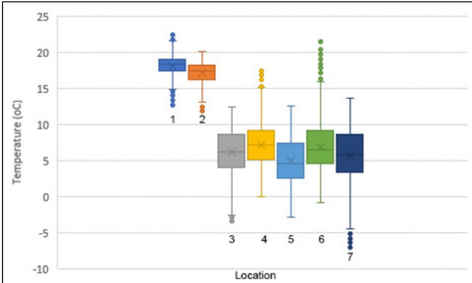
Fig 94: Interquartile temperature ranges (°C) from below the ceiling (BC) to the exterior for January/February 2016, when there was 100mm of glass fibre insulation
