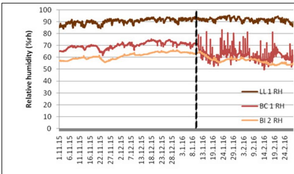
Fig 28: Occupancy (dotted line) and its effects on relative humidity (%) below the ceiling (BC), below the insulation (BI) and at low level (LL) within the roof
