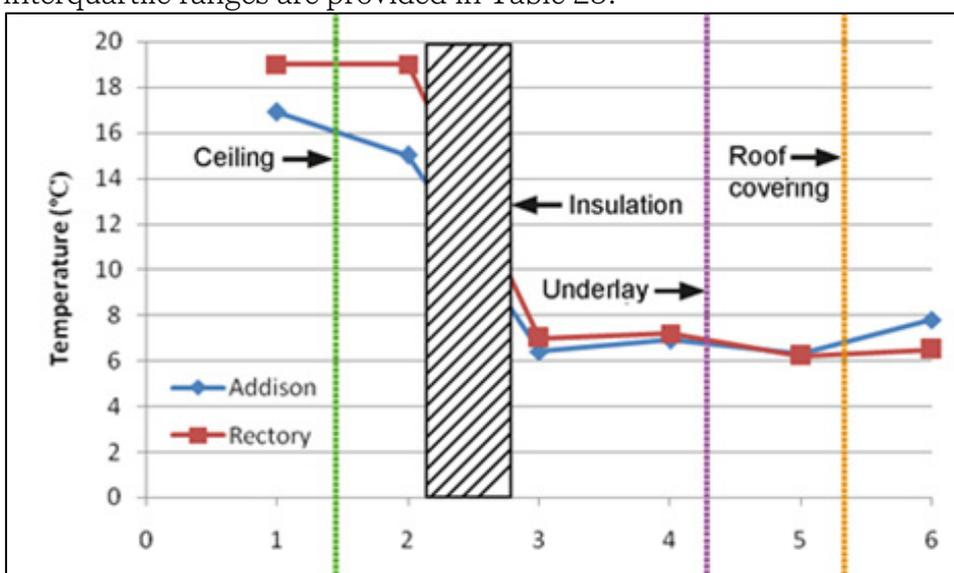
Fig 142: The median temperature gradients across the roof from the room (1) to the exterior (6) during the first week of January 2017
