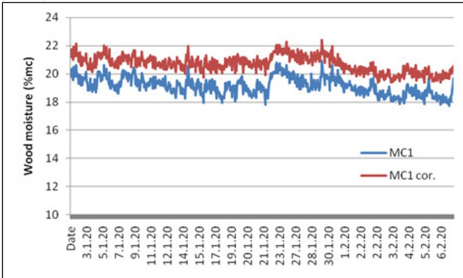
Fig 139: January/February 2020 corrected and measured moisture content data (calculated from resistance). The corrected readings are higher because the surface temperature of the wood is low
