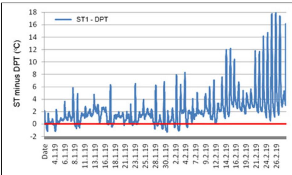
Fig 122: January/February 2019 condensation events (below red line) for the south slope of the roof
