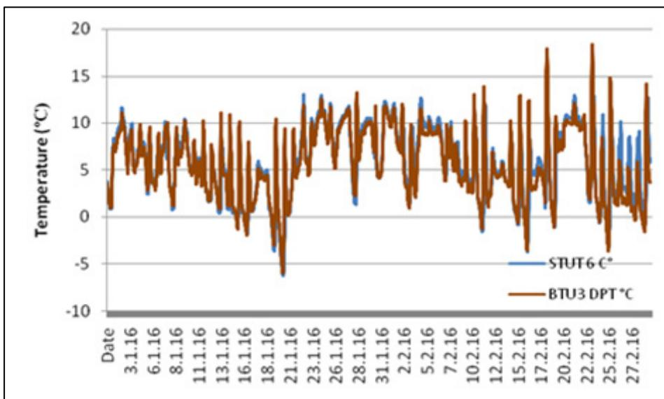
Fig 25: A comparison of dew point (BTU3 DPT) with surface temperature on the underside of the tiles (STUT6) for January/February 2016, showing that they overlap. Condensation would be a frequent event
