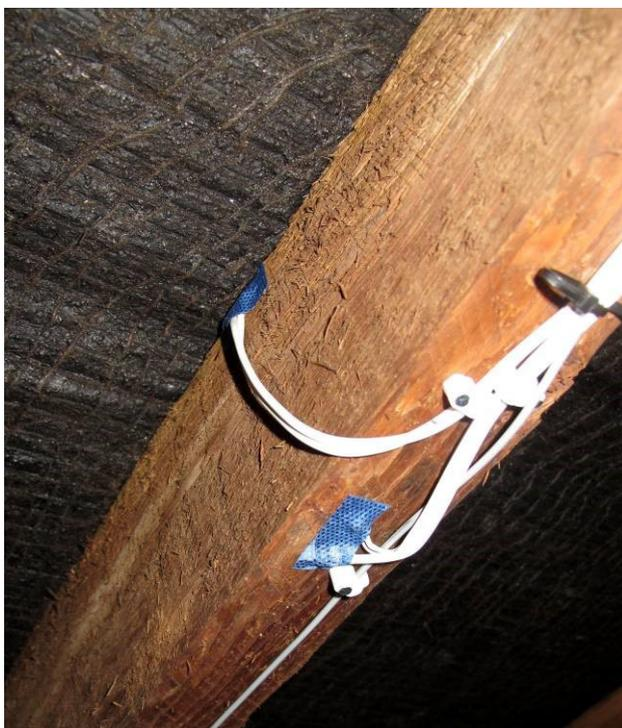
Fig 138: Wood moisture content sensors MC1 (upper nearest underlay) and MC2 (lower)
