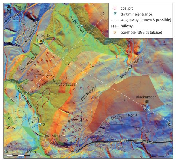
Figure 19: Schematic plan of coal workings at Gibside and environs. [background image lidar DTM 2018 © Historic England; source Environment Agency]
