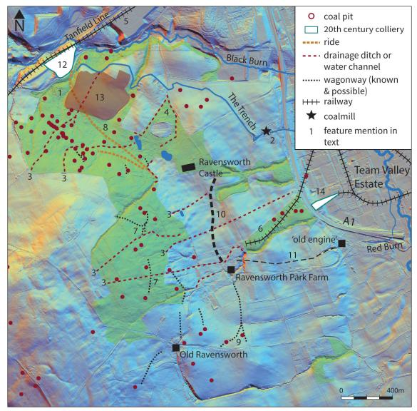
Figure 21: Schematic plan of coal workings at Ravensthorpe Gibside and environs. [background image lidar DTM 2018 © Historic England; source Environment Agency]
