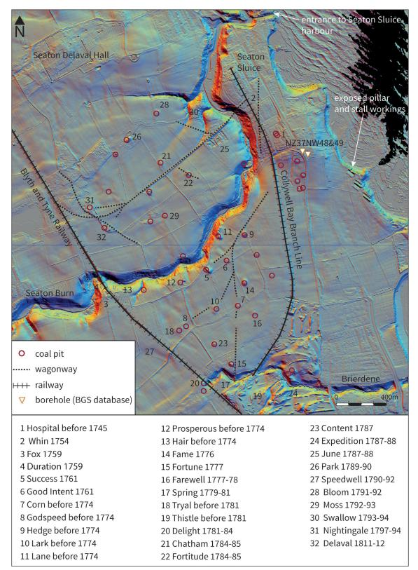
Figure 18: Schematic plan of coal workings at Hartley, with additional information from Tomlinson 1915. Pits are numbered chronological by date sunk. Not all pits are named and not all named pits were recorded by this project. [background image lidar DTM 2018 © Historic England; source Environment Agency]
