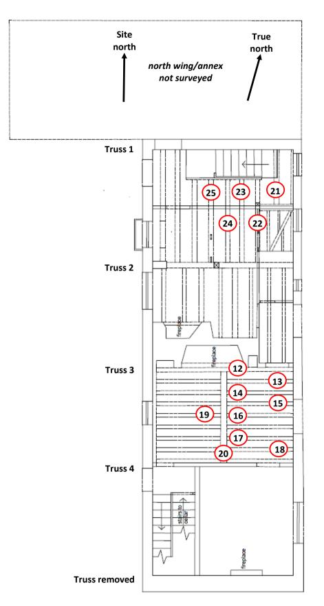
Figure 3b: Plan at ground-floor level to show the locations of the sampled timbers (after Rebecca Lane 2021)
