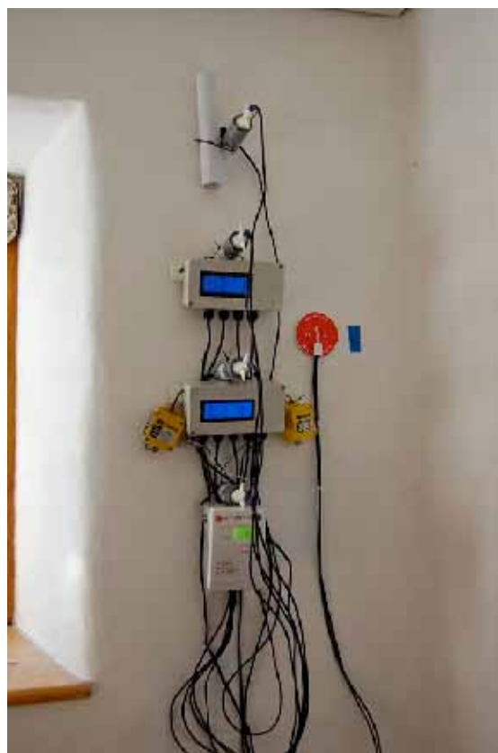
Figure 35. Interstitial, U-value and IAQ monitoring set up at The Firs, Riddlecombe, 2012.
