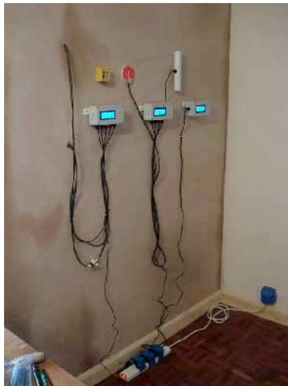
Figure 50. Interstitial, U-value and IAQ monitoring set up at Mill House, Drewsteignton, 2012.
