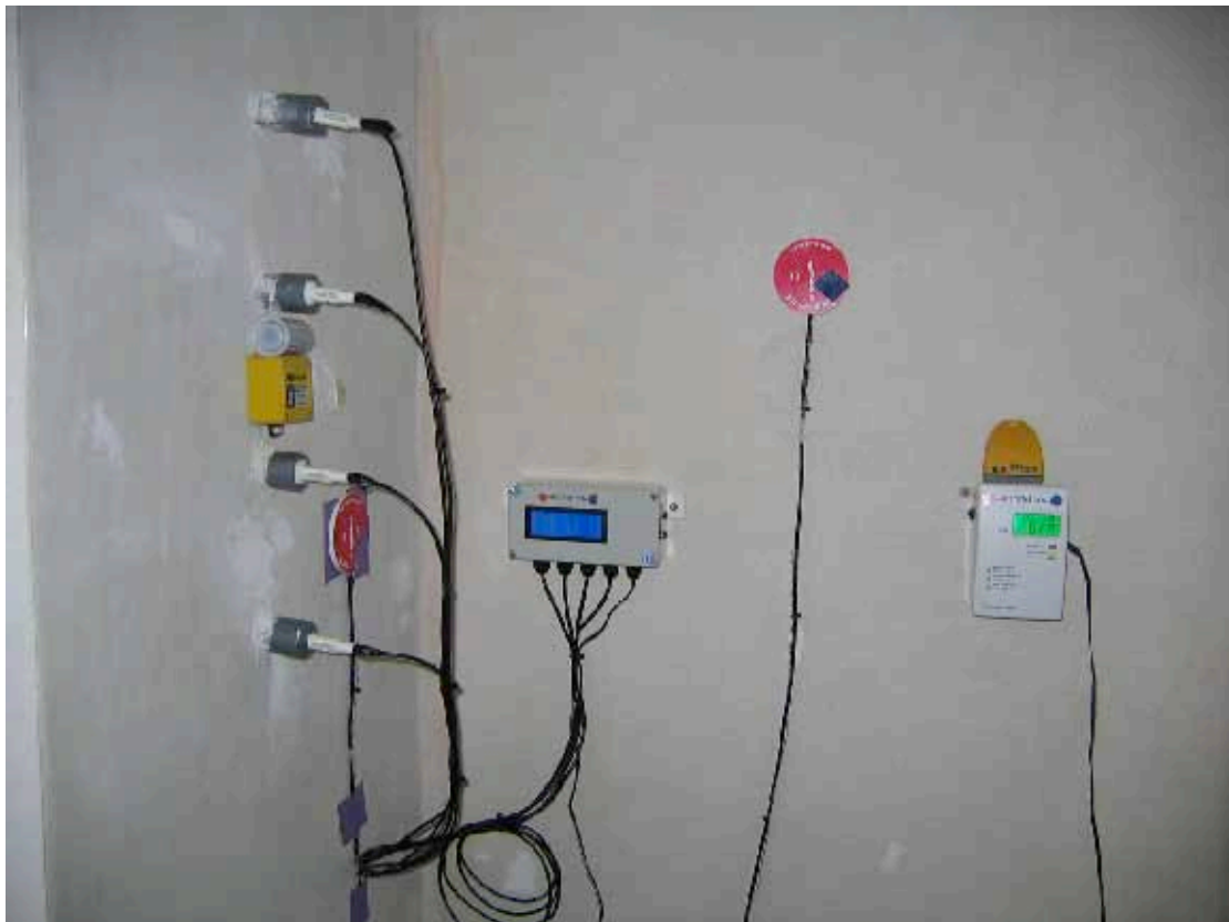
Figure 17. Interstitial, U-value and IAQ monitoring set up at Abbeyforegate, Shrewsbury, 2012.
