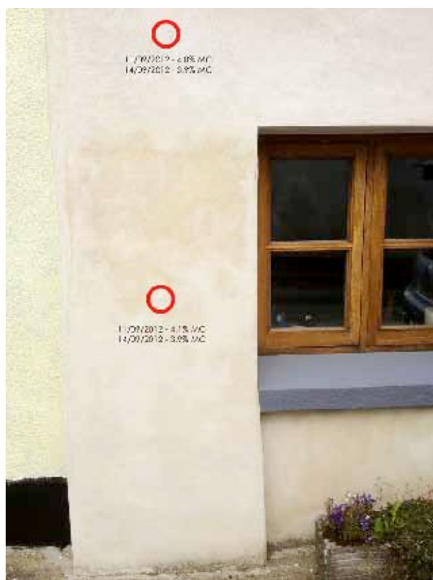
Figure 41. Moisture content resistivity probes in external wall face, The Firs, Riddlecombe, September 2012.
