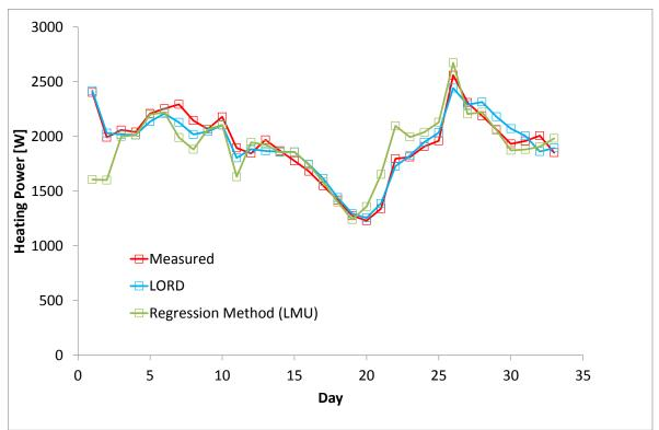
Figure A17: Comparison of measured and predicted daily average heating power for the post-intervention co-heating test.
