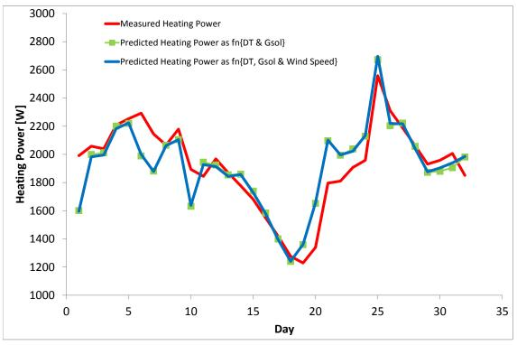
Figure A14: Post-intervention case. Measured and predicted heating power using (a)  $\Delta T$  and Gsol as the independent variables (Equation A1) and (b)  $\Delta T$ , Gsol and wind speed (Equation A4). Note: the line for the two predictions of heating power are effectively co-incident.
