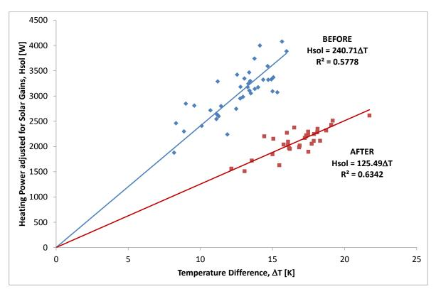
Figure A12: LMU method - heating power adjusted for solar gains plotted against temperature difference for the before and after co-heating tests.
