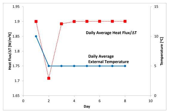
Figure A5: Demonstration of the effect of the step change in external temperature on the daily average value of the heat  $flux/\Delta T$ .
