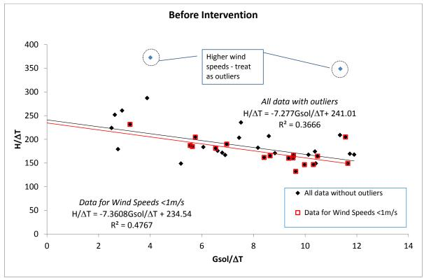
Figure A10: Before Intervention.  $H/\Delta T$  vs.  $Gsol/\Delta T$  plot for the daily average values from the co-heating test. The linear regression fits for all the data and only the data for wind speeds less than 1m/s are shown. The intercept on the  $H/\Delta T$  axis gives the whole house heat loss coefficient value ( $\Omega$ -value) and the slope the solar gain factor (gA-value).
