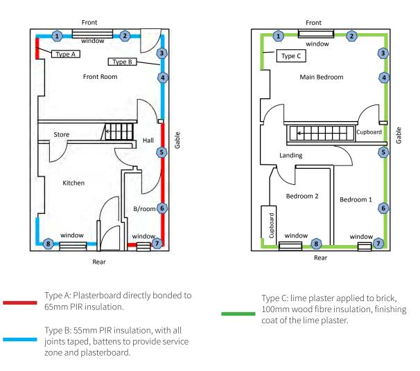
*Figure 4: Location of the two internal wall insulation systems – left: ground floor with PIR; right: first floor with wood fibre system.*
