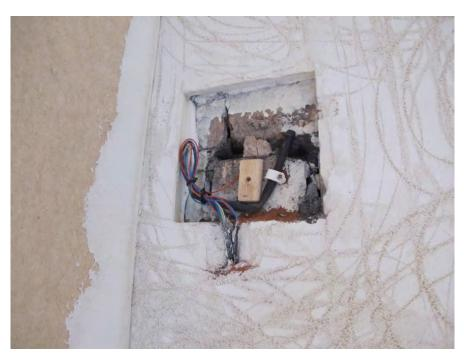
Figure 28: Relative humidity/temperature and resistance sensors fixed on the wall prior to the installation of internal wall insulation
