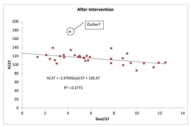
Figure A11: After Intervention.  $H/\Delta T$  vs.  $Gsol/\Delta T$  plot for the daily average values from the co-heating test. The linear regression fit for all the data without the outlier is shown.
