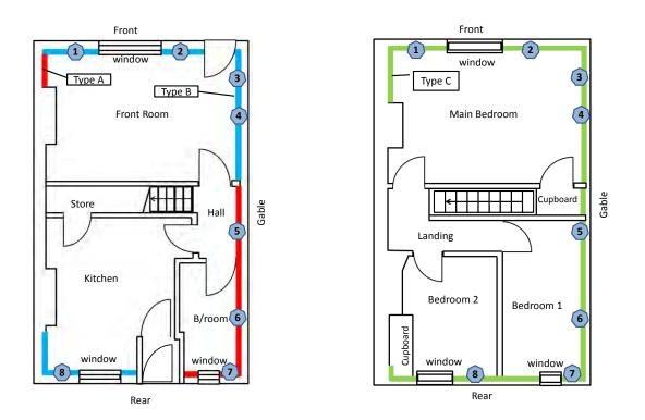
Figure 27: Plan of the monitoring locations with two sensors in each location positioned at low and high level
