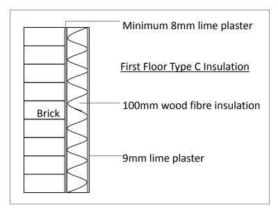
Figure 3: First floor insulation system
