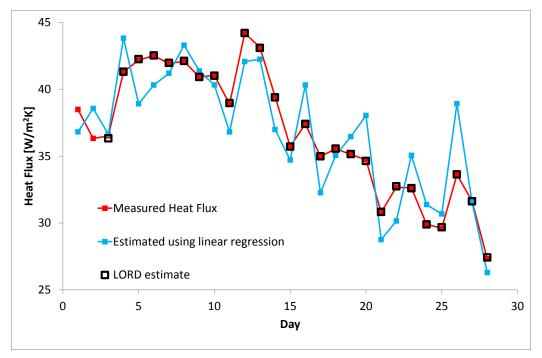
Figure A9: Comparison of the daily average heat flux estimates using linear regression and LORD with the simulated measured values for the simulated 9" brick wall. Note that the LORD estimates overlap the measured heat flux values.
