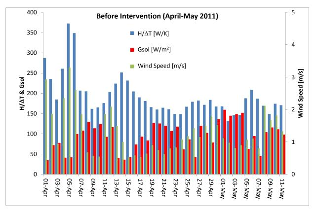
Figure 13: Before Intervention. The daily average values of H/ΔT, Gsol and wind speed during the co-heating test.
