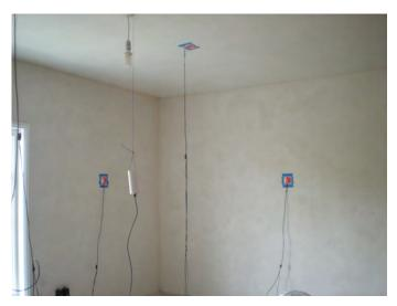
Figure 5: In situ U-value measurements in main bedroom: front elevation, gable wall and ceiling.
