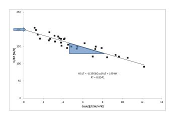
Figure A2: Example of X-Y plot of co-heating test data (Siviour analysis). The intercept of the linear regression line is the whole house heat loss coefficient and the slope is the solar gain factor
