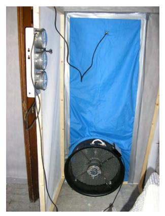
Figure 7: Blower door assembly for building pressurisation test.
