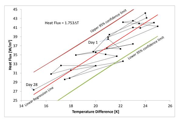
*Figure A6: Daily average heat flux vs. temperature difference for simulated data using varying external temperature with 9" brick wall. The linear regression line, the slope of which gives the U-value, and the confidence limits.*
