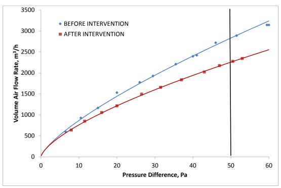
Figure 11: Building pressurisation test results before and after improvement measures for New Bolsover
