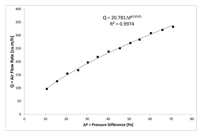
Figure 8: Example of building pressurisation test data with power law curve fit
