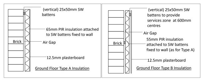
Figure 2: Ground floor insulation systems
