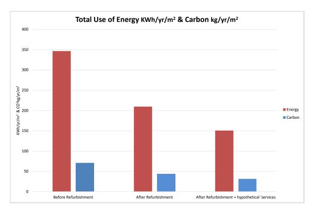
Figure 32: Total energy and carbon use before and after refurbishment, including installation of hypothetical services
