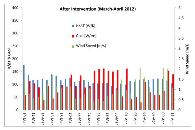
Figure 14: After Intervention. The daily average values of H/ΔT, Gsol and wind speed during the co-heating test.
