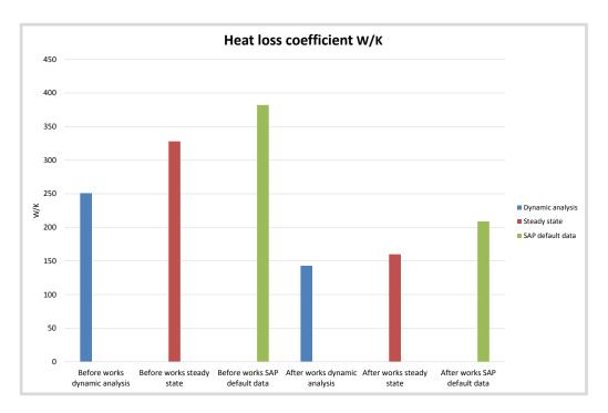
Figure 30: Range of heat loss coefficients depending on the method of analysis
