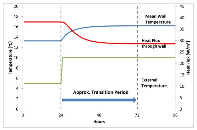
Figure A4: Simulated results for a 9" brick wall for a step change in external temperature, demonstrating the effect of thermal storage in the wall on mean wall temperature and heat flux through the wall.
