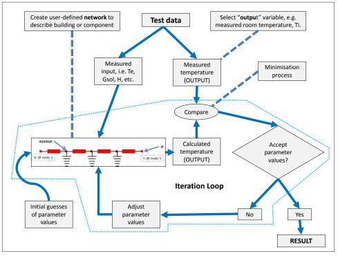
Figure A8: Parameter identification principle.
