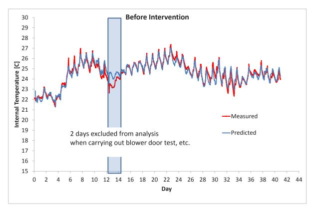
*Figure A16: The predicted and measured output variable (average room temperature in the house)*
