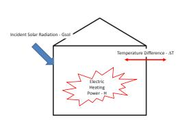
Figure A1: Schematic diagram of main parameters for analysis of co-heating test data using simplified analysis
