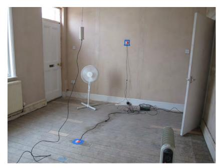
Figure 26: Co-heating test set-up
