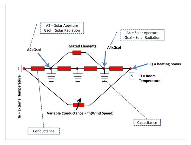
Figure A15: House modelled as a network of conductances and capacitances.
