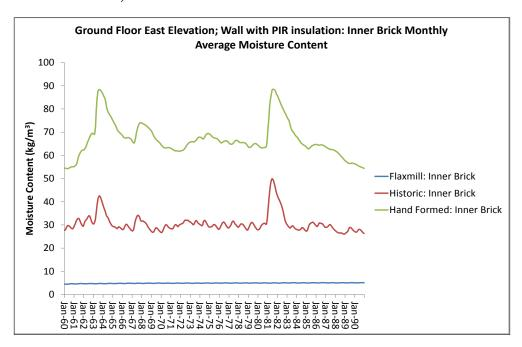
Figure 23: Ground Floor East Elevation; wall with PIR insulation: inner brick monthly average moisture content
