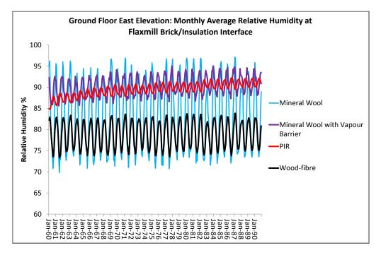
Figure 32: Ground Floor East Elevation: monthly average relative humidity at Flaxmill brick/insulation interface
