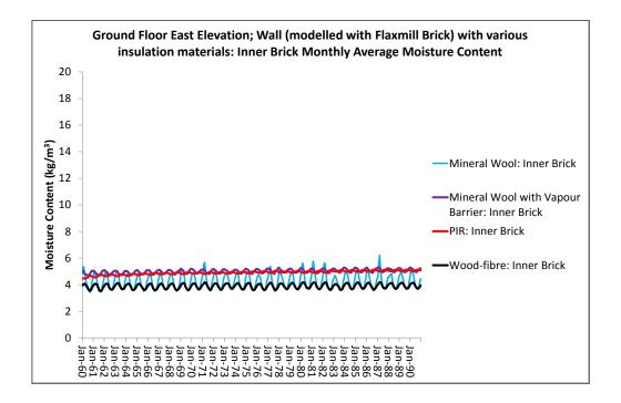
Figure 31: Ground Floor East Elevation; wall (modelled with Flaxmill brick) with various insulation materials: inner brick monthly average moisture content
