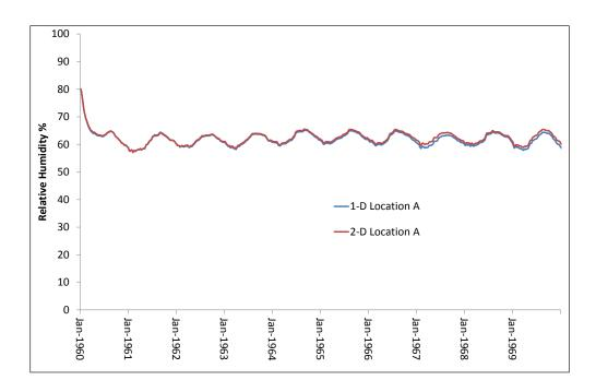
Figure 11: Comparison of 1-D and 2-D simulations of case 1 brick wall only
