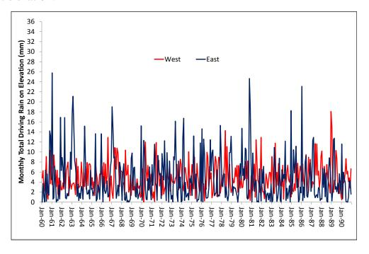
Figure 5: Monthly totals of driving rain calculated for each elevation
