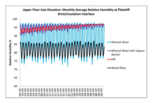
Figure 34: Upper Floor East Elevation: monthly average relative humidity at Flaxmill brick/insulation interface
