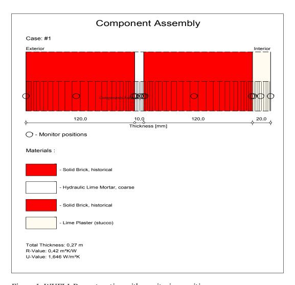
Figure 1: WUFI 1-D construction with monitoring positions
