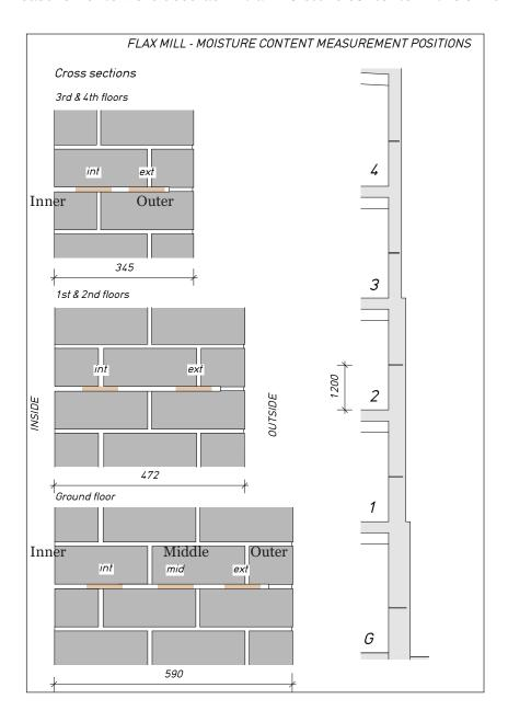
Figure 3: Wall construction of the five floors of Shrewsbury Flaxmill Maltings, showing 1-D simulation profiles in beige
