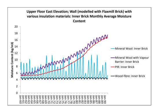
Figure 33: Upper Floor East Elevation; wall (modelled with Flaxmill brick) with various insulation materials: inner brick monthly average moisture content
