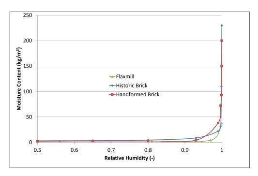
Figure 4: Moisture absorption curves of the three bricks
