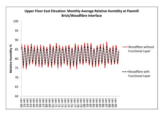
Figure 35: The effect of the functional layer in the wood-fibre insulation sustem
