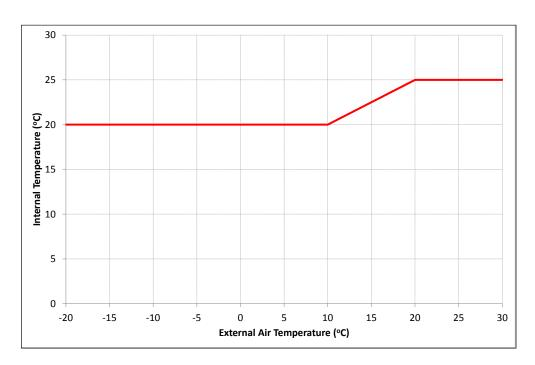
Figure 6: Variation of internal temperature with external temperature
