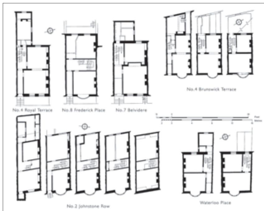
Figure 23 (above, left) Seaside houses employed the types of plan found in towns throughout England, but instead of being family homes with definite functions for each room, these were used flexibly to accommodate visitors.
