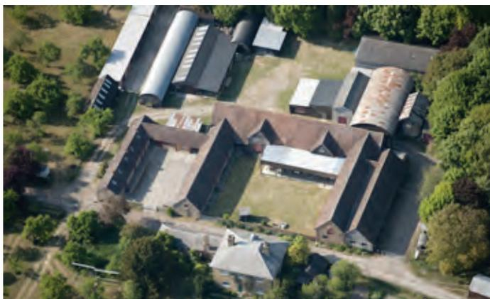
This F-plan farmstead in north Buckinghamshire has a detached house (at bottom of picture) facing away from the yard, which is dominated by its threshing barn with gabled porches to its two threshing floors. The additional cattle yard to the left of the photograph completes the overall F-shaped plan. Photo © English Heritage NMR 26954/020
