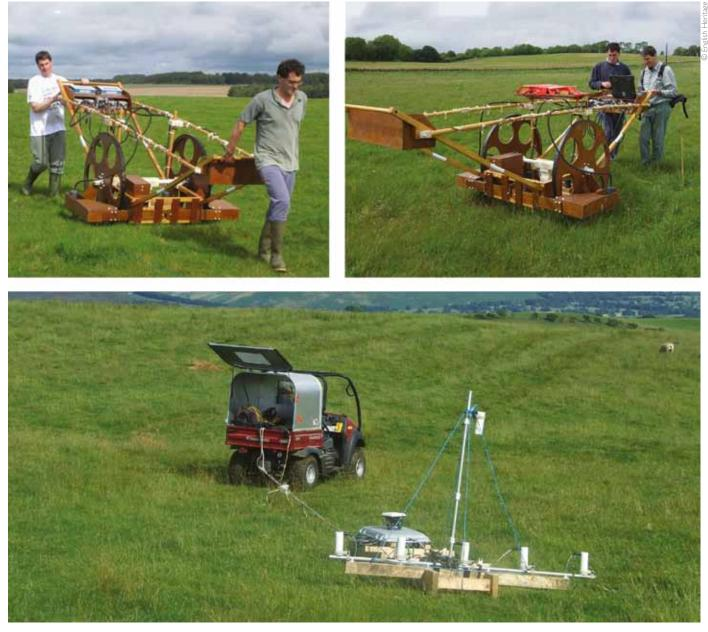
Development of the system, from hand-pushed to vehicle-towed. *Top left:* Hand Pushed Scintrex 4 sensor system, *top right:* Hand pushed system with GPS for "grid less" survey. *Bottom:* Vehicle towed system with GPS and 6 Geometrics sensors
