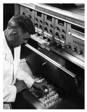
**Fig 19.** Geoff Bradburn loading counting vials into a Packard model 337 Liquid Scintillation Spectrometer at AERE Harwell. (© NDA, reproduced with permission from the NDA)
