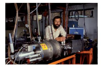
**Fig 17**. Robert Hedges undertaking maintenance on the first accelerator mass spectrometer at the Oxford Radiocarbon Accelerator Unit. (© ORAU)
