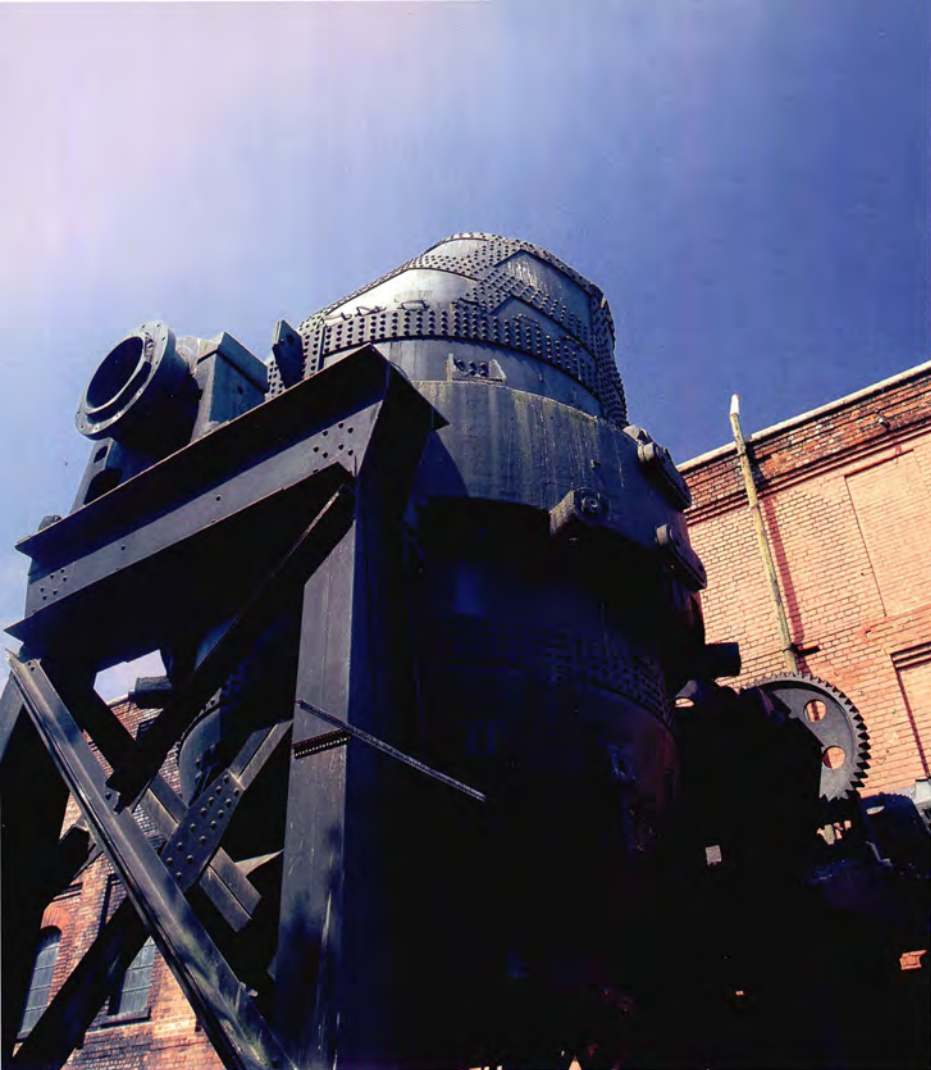
Fig 9 The Bessemer converter introduced bulk steel production to Sheffield. This rare survival comes from Workington and is on display at the Kelham Island Museum. [AA022440]
