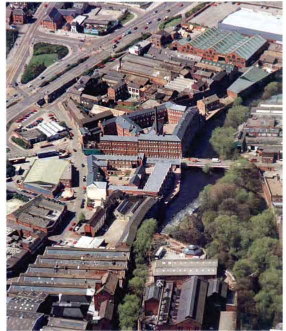
Fig 71 (top right) The landscape of Sheffield's metal trades: a view of the Kelham Island area showing a saw and file factory, a foundry, Cornish Works, and steel and cutlery works. The weir across the River Don feeds water into a headrace, a reminder that water power was once important even in Sheffield itself. [NMR 17567-11]
