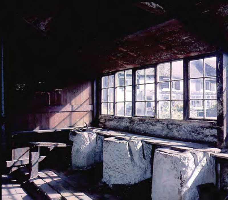
Fig 48 (bottom) The interior of the file workshop at 11 High Street, Ecclesfield. The files were cut on the stone blocks set beneath the windows, which could be secured at night by lowering the internal shutters. The room contained hearths for working the metals. [FF000791]
