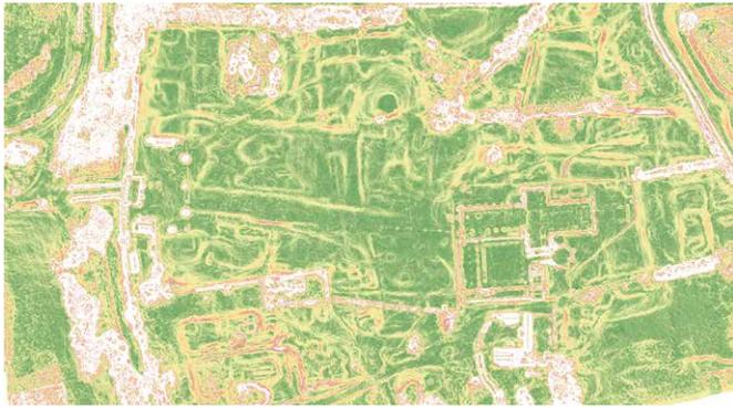
Slope analysis of the filtered digital elevation model. Flatter areas are shown in green, intermediate slopes in yellows, steeper slopes in shades of red.
