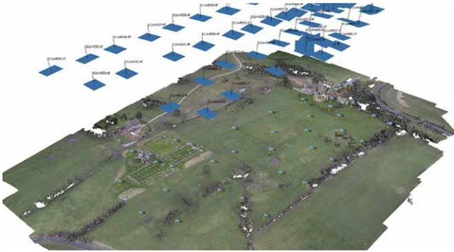
The dense point cloud generated from the aerial photography. Camera positions can be seen above the point cloud, while the small flags denote ground control points.
