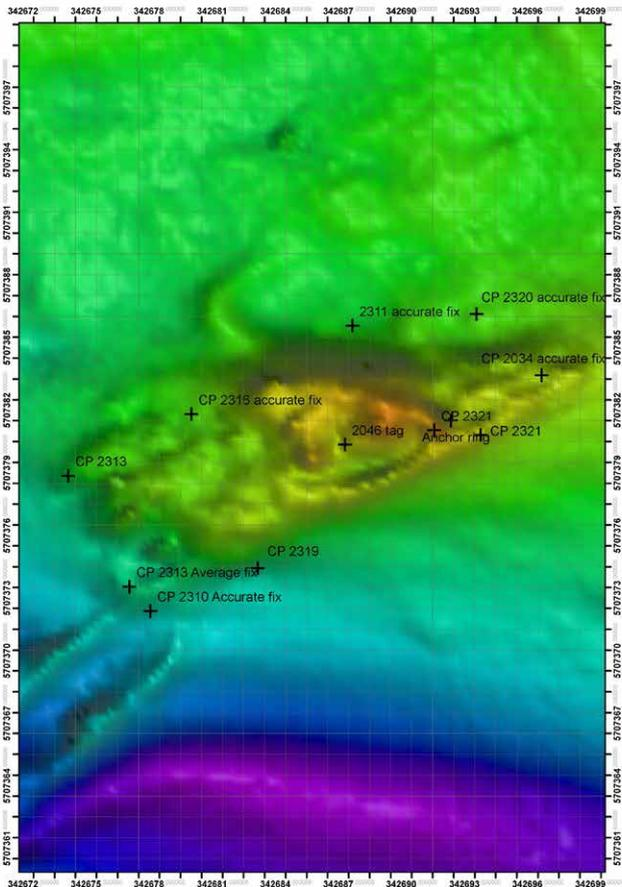
Multibeam bathymetry image of the presumed site of the *London*. The large raised area in the centre of the site represents archaeological deposits from the wreck. Some of the linear features visible here are disarticulated structural components of the ship. To the bottom left the remains of a more recent vessel can be seen.
