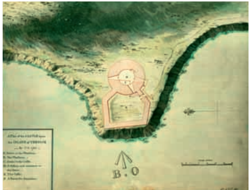
Figure 33 In 1715 Christian Lilly surveyed Cromwell's Castle and found that the structure, only 60 years old, was still serviceable though in need of repairs. The plan shows the attached gun platform that was reworked in the 1740s.
