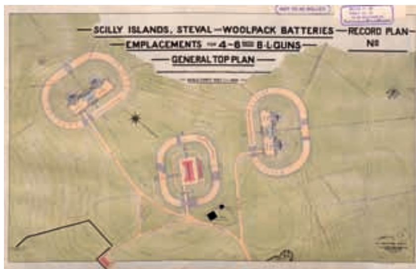
Figure 61 This survey drawing of 1902 shows the completed pair of gun batteries with the barracks block between. Below the barracks can be seen the tower of the signal station – a refurbished old windmill and not a gun tower of the early 19th century. The site of the second old windmill is shown a short distance to the left.
