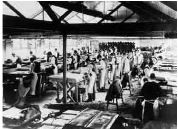
Fig 31 (above, left) Manfield's rough-stuff department, with revolution presses for bottom-stock cutting, in the 1920s. At this stage, the different components of boots and shoes were carried around the factory in wicker baskets, which can be seen in the foreground. Pattern racks can be seen against the far wall. [Northampton Museums and Art Gallery]
